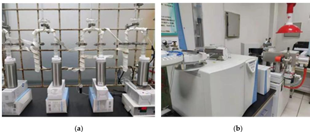
**Figure 3.** The pictures in the experiment process. (a) Moisture extraction equipment; (b) Isotope analysis equipment.
