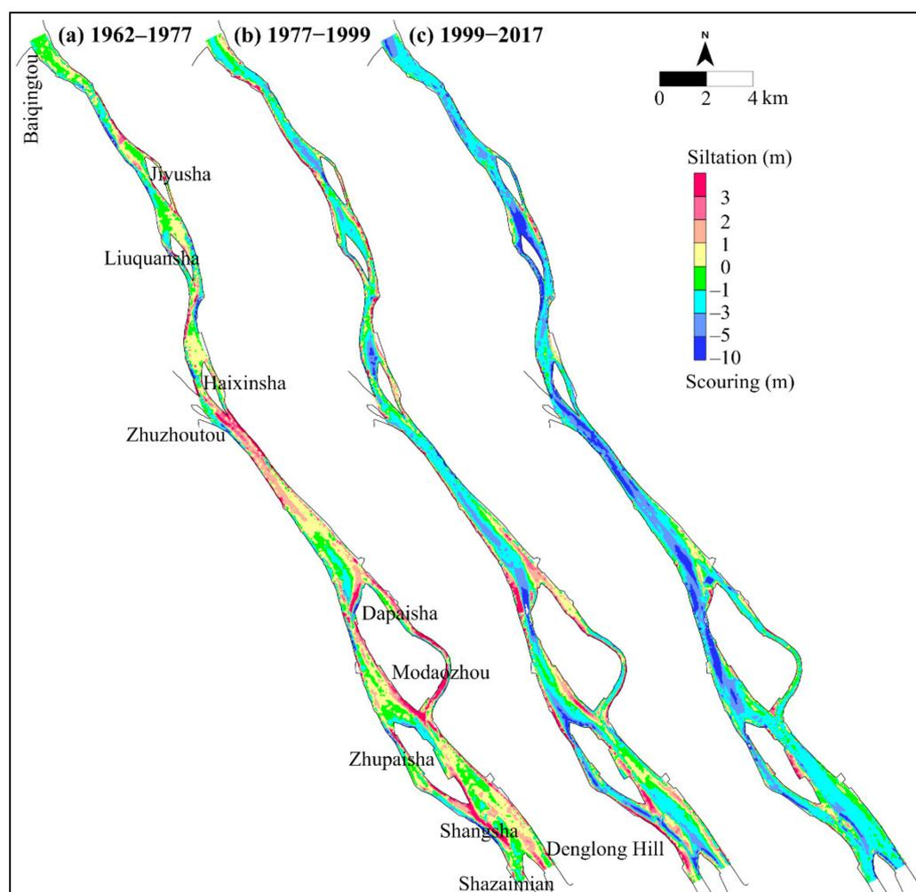
**Figure 5.** Maps of scouring and siltation along the channel during different decades. (a) 1962–1977, (b) 1977–1999, and (c) 1999–2017.
