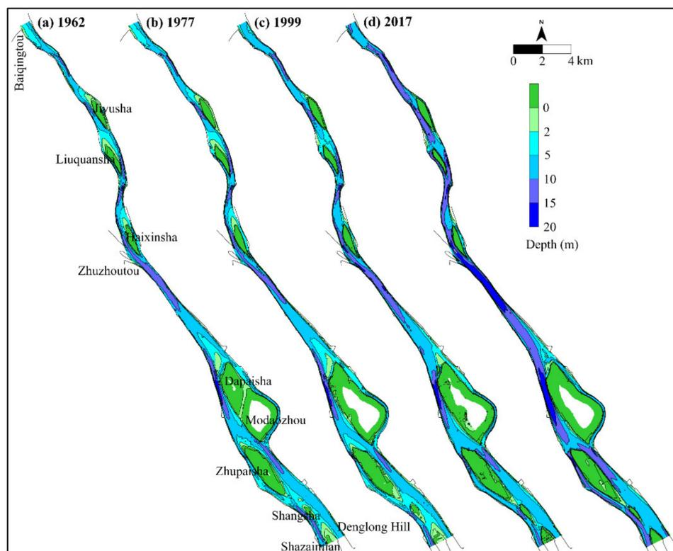
**Figure 2.** Bathymetry of the Modaomen Channel in (a) 1962, (b) 1977, (c) 1999, and (d) 2017.
