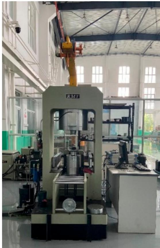
**Figure 3.** RMT-301 rock and concrete mechanics experimental system.
