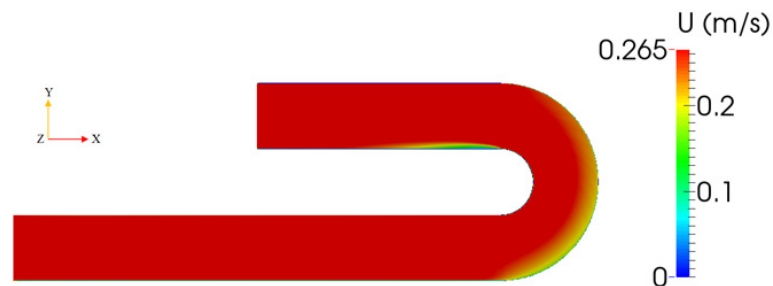
Figure 7. The distribution of water surface velocity (Realizable k-\epsilon ).
