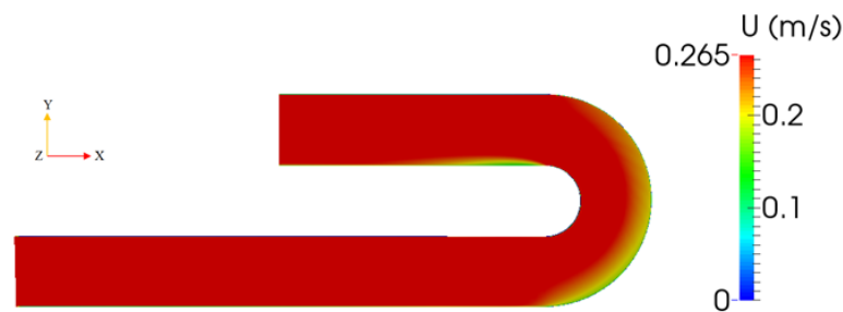
Figure 6. The distribution of water surface velocity (Standard k-\epsilon ).
