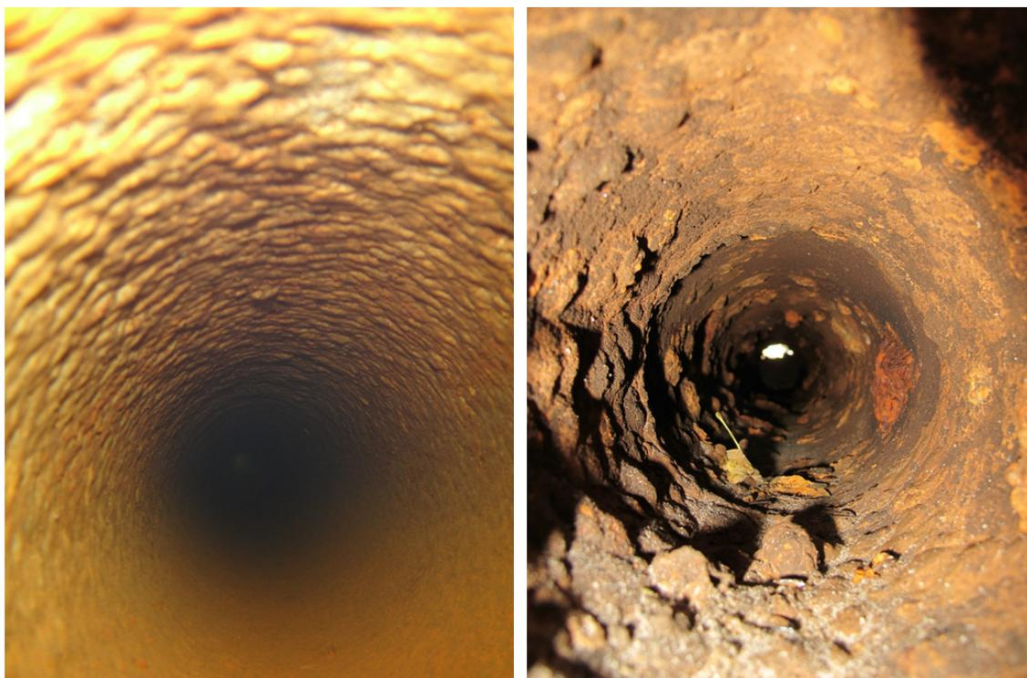
**Figure 1.** View inside drinking-water pipes; **left** side with small-scale incrustations and biofilm layer as a habitat for invertebrates (ND = 100); **right** side with corrosion of a cast iron pipe (ND = 80).
