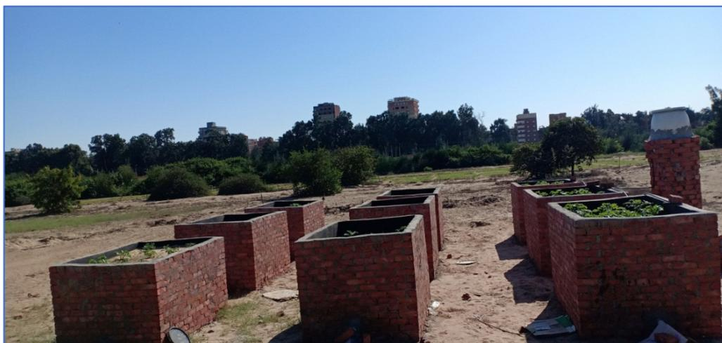
**Figure 2.** Nine experimental lysimeters, each 1.5 m long, 1.0 m wide, and 1.0 m high.
