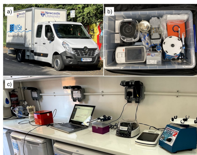
Figure 1. (a) Mobile laboratory in the back of a van; (b) the equipment items needed for onsite marker gene quantification inside a suitcase for transportation, and (c) the equipment items set up on the bench of the mobile laboratory, from left to right: vacuum pump, filtration unit, qPCR instrument, laptop computer, pipettes and tips, centrifuge, fluorometer, and vortex with adapter.
