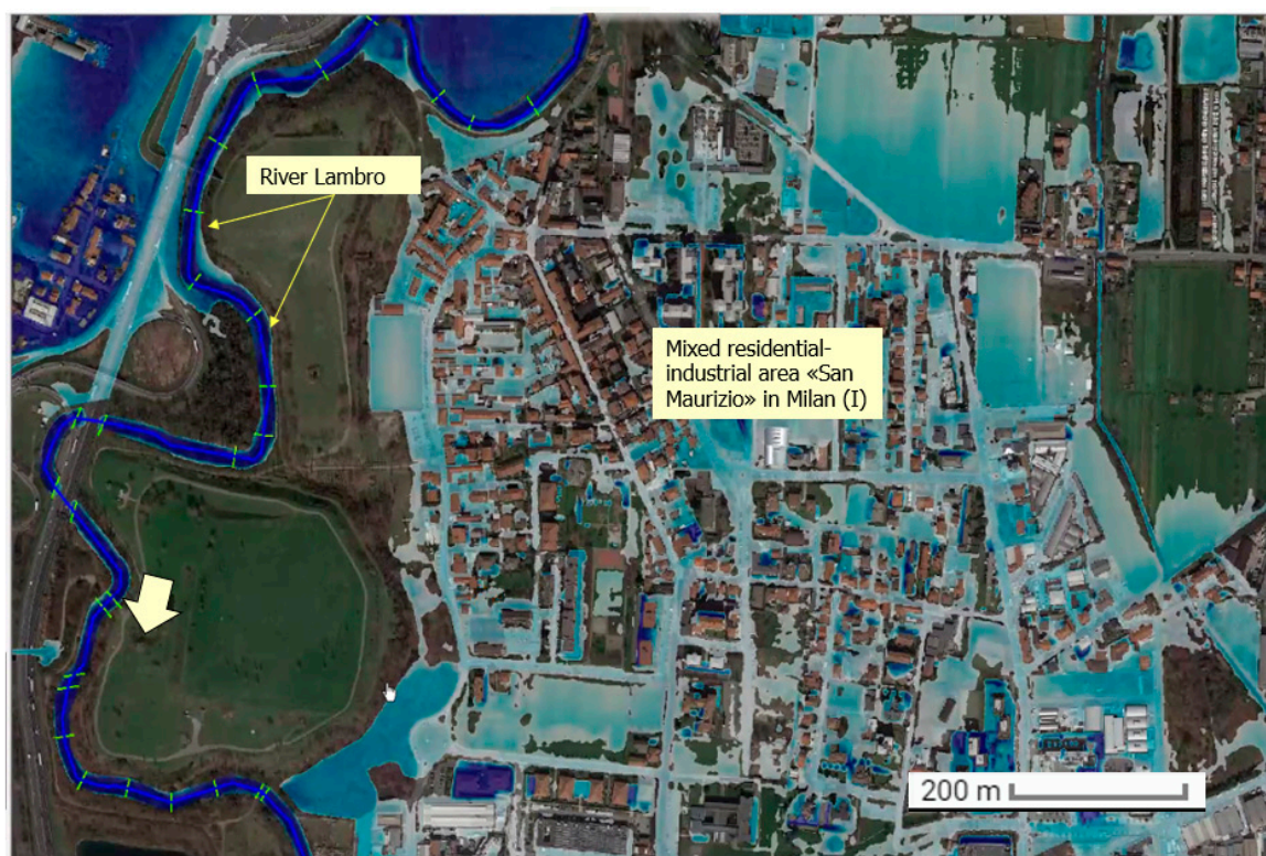
Figure 7. Rivers will flood urban areas as well; such areas must be equipped and prepared to minimize damages (Lambro river at San Maurizio al Lambro in Milan (I), in a simulation of a T_{R200} event, by kind concession of Alessandro Balbo).
