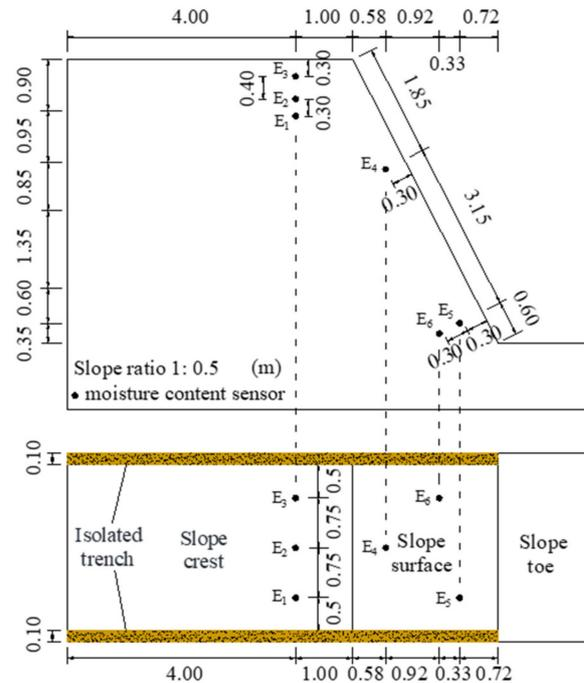
Figure 4. Schematic diagram of moisture sensor layout.
