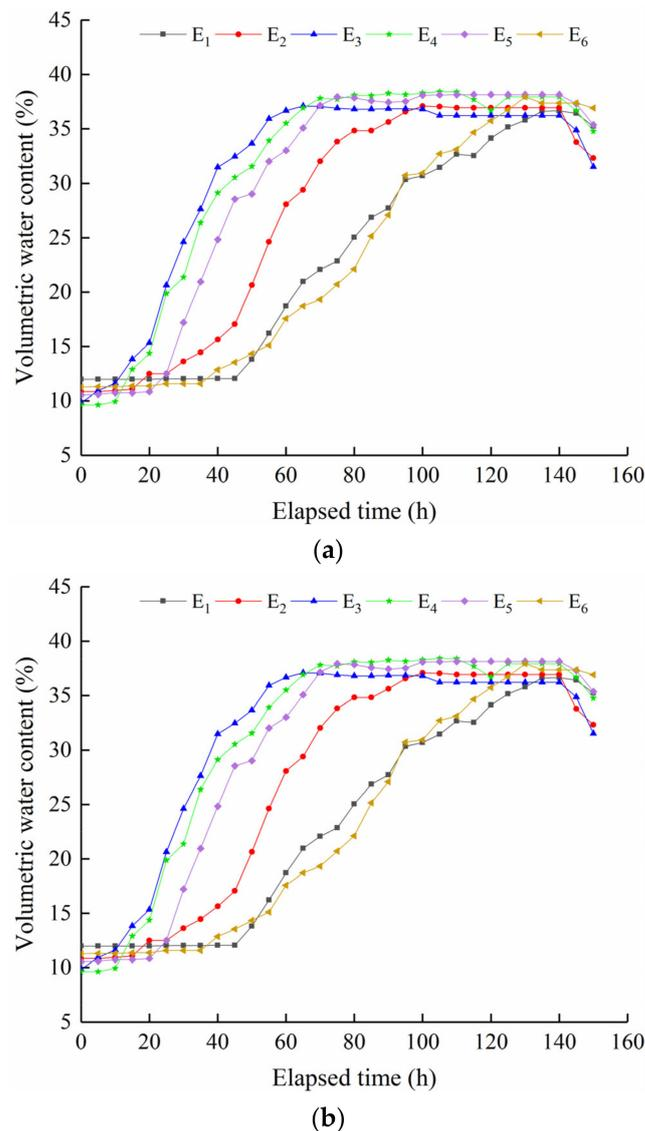
**Figure 8.** Change curves of volumetric water content at measuring points: (a) under heavy rainfall; (b) under rainstorm.
