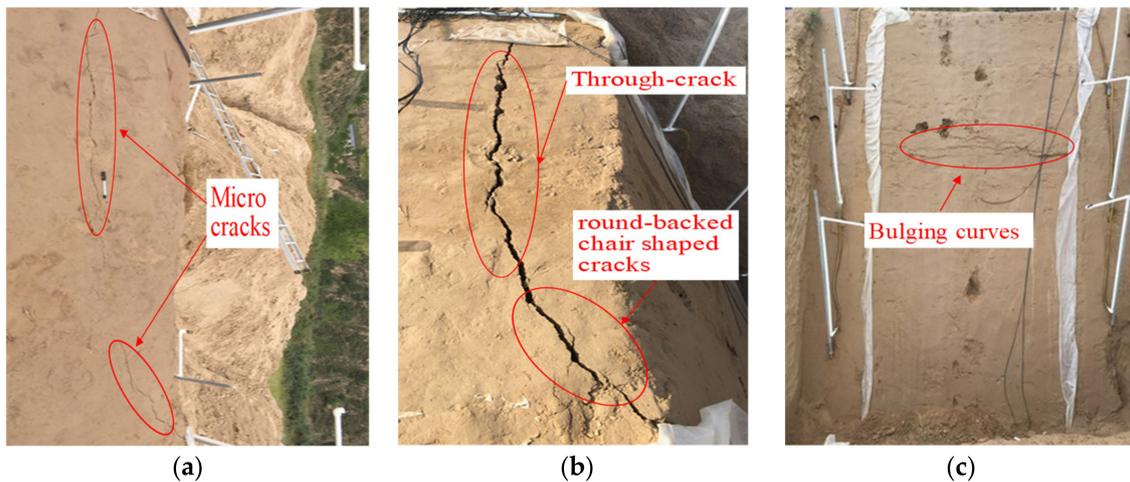
**Figure 6.** Cracks of the slope under heavy rainfall: (a) microcrack growth; (b) transverse penetration of crack at the slope crest; (c) bulging curves at the slope surface.
