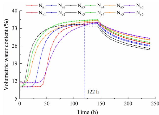
**Figure 12.** Change curves of volumetric water content in the two numerical simulations.
