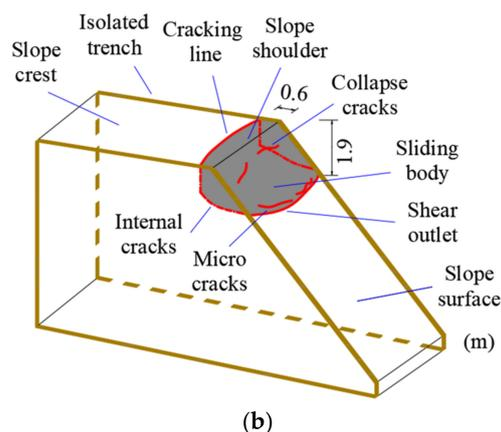
**Figure 10.** Schematic diagram of failure mode under rainfall of the local slope: (a) heavy rainfall, (b) rainstorm.
