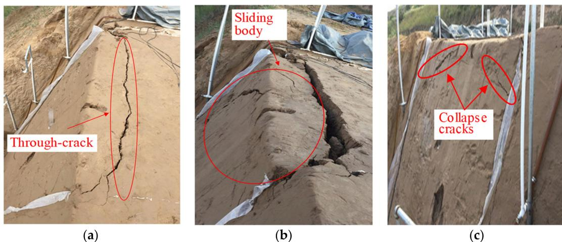
**Figure 7.** Cracking of the slope under rainstorm: (a) through-crack at the slope crest; (b) sliding body of the slope; (c) collapse cracks at the slope surface.
