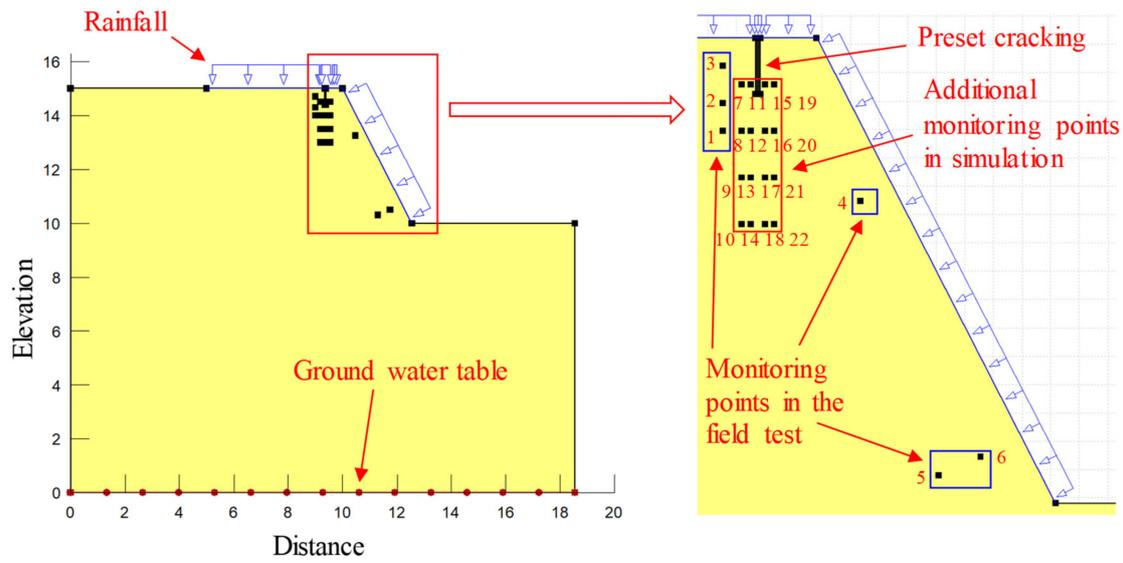
**Figure 11.** Monitoring points of numerical models under simulated rainstorm.
