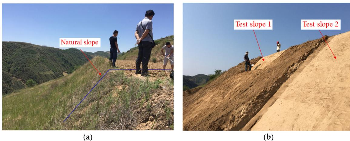
**Figure 2.** Test slope: (a) natural slope, (b) test slope after trimming.
