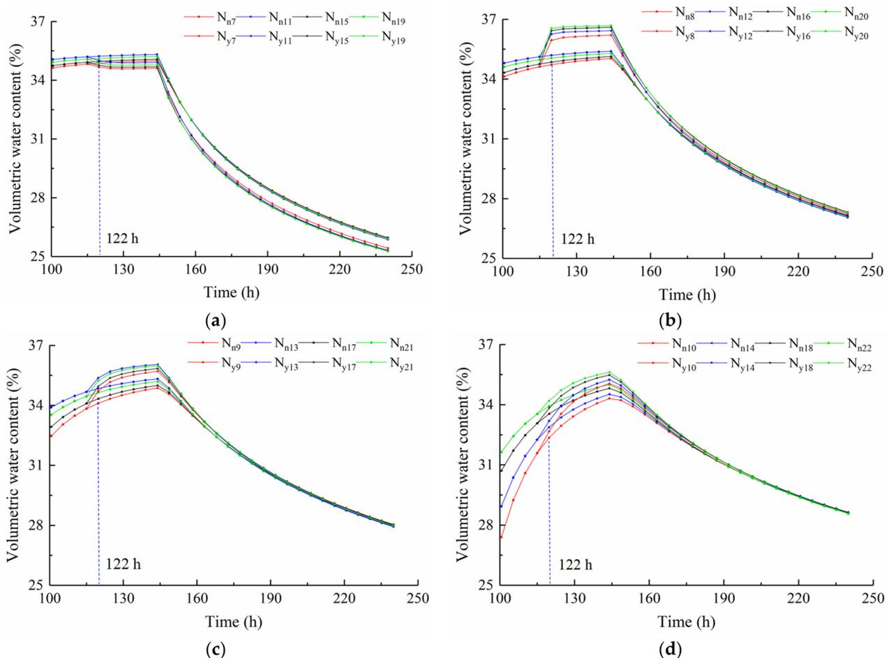
**Figure 13.** Curves of volumetric water content in additional monitoring points in the two numerical simulations: (a) upper points; (b) middle points; (c) lower points; (d) bottom points.
