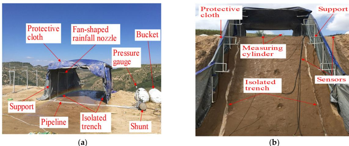
Figure 5. Rainfall on test site: (a) rainfall on the slope crest; (b) rainfall on the slope surface.
