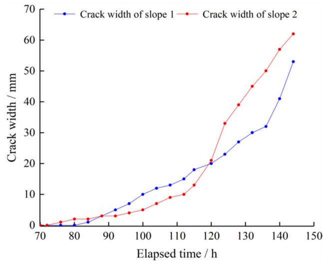
Figure 9. Curves of crack width with time in test slopes.
