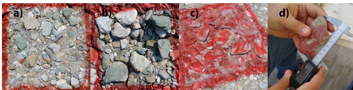
**Figure 3.** Grid sampling method of 1 m<sup>2</sup> [8] applied in grids of inhomogeneous bed composition (a–c) and axes measurements at laboratory facilities (d).
