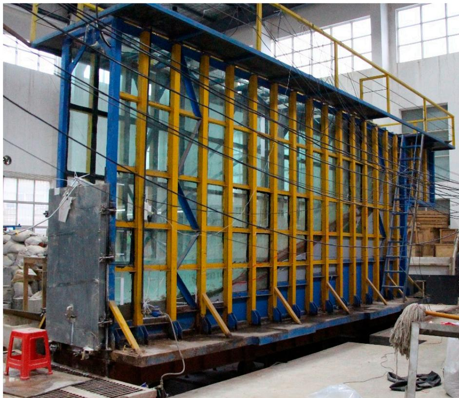
Figure 4. Landslide model test system.
