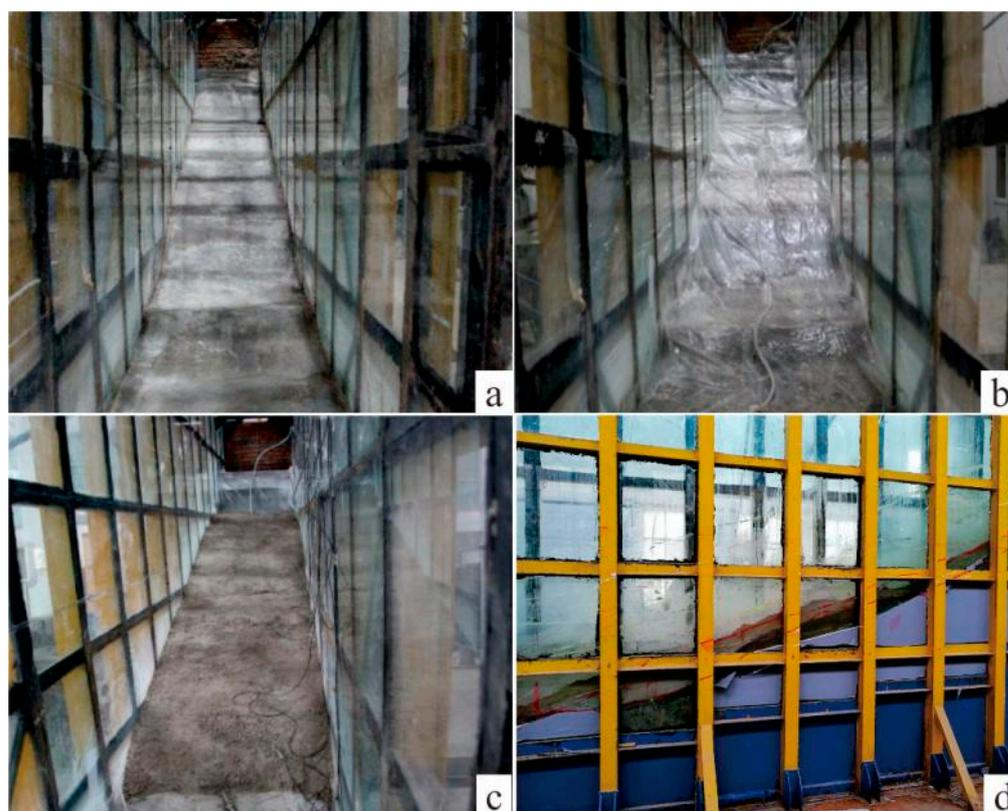
**Figure 7.** Construction of the physical simulation models: (a) Slide bed; (b) Slide surface; (c) Slide mass; (d) Entire model.
