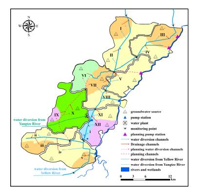
Figure 4. Water resources allocation system network diagram in Guantao County.
