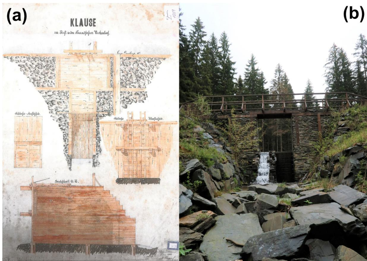
**Figure 11.** The splash dam on Splavský creek: (a) a historical technical drawing from 1863, and (b) the current state after a 2014 reconstruction.
