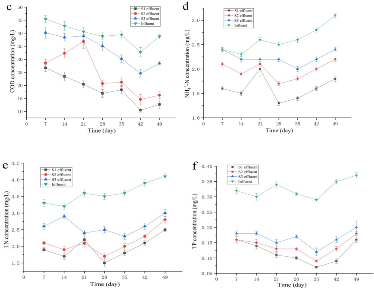
**Figure 4.** Influent and effluent temperature in S1–S3 (a); influent and effluent pH in S1–S3 (b); influent and effluent COD concentrations in S1–S3 (c); influent and effluent  $\text{NH}_4^+\text{-N}$  concentrations in S1–S3 (d); influent and effluent TN concentrations in S1–S3 (e); influent and effluent TP concentrations in S1–S3 (f).
