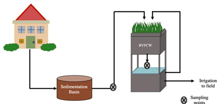
**Figure 1.** Recirculating vertical flow constructed wetland schematic.
