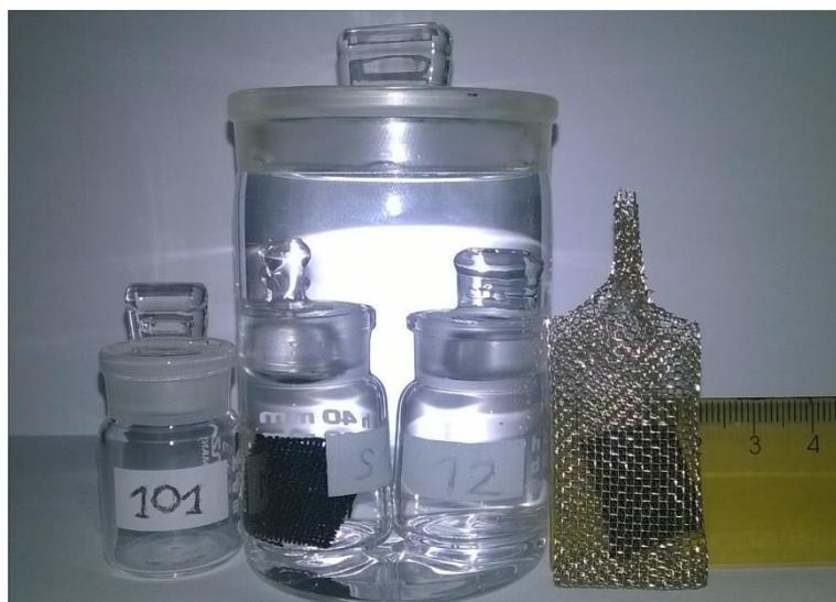
**Figure 1.** Weighing bottles filled with UPW for the transport of passive samplers and stainless steel casing with ACFs.
