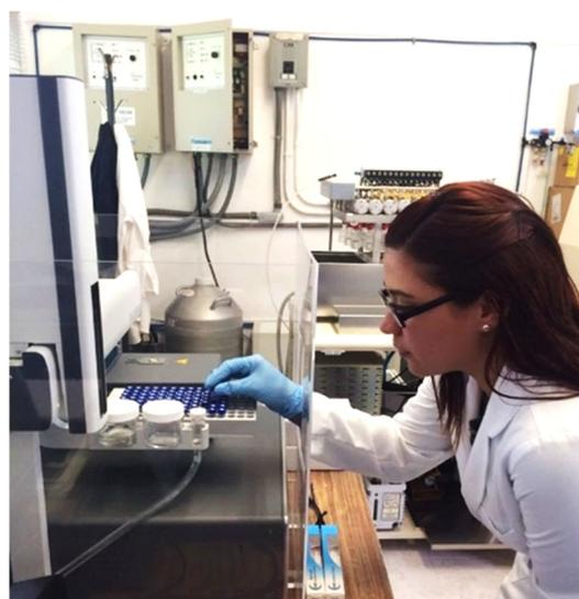
**Figure 3.** Analyzing stable isotopes ( $\delta^{18}\text{O}$ ) samples at the Isotopic Hydrologic Laboratory (Laser analyzer Cavity Ringdown Spectrometer L2110-i Isotopic  $\text{H}_2\text{O}$  Picarro with high precision vaporizer A0211).
