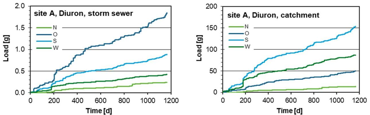
**Figure 7.** Cumulative exposure-dependent diuron load of all building façades in connection with the storm sewer (**left**) and of all façades of site A (**right**). The scenario-based simulations cover 3 years starting with the construction of the site.
