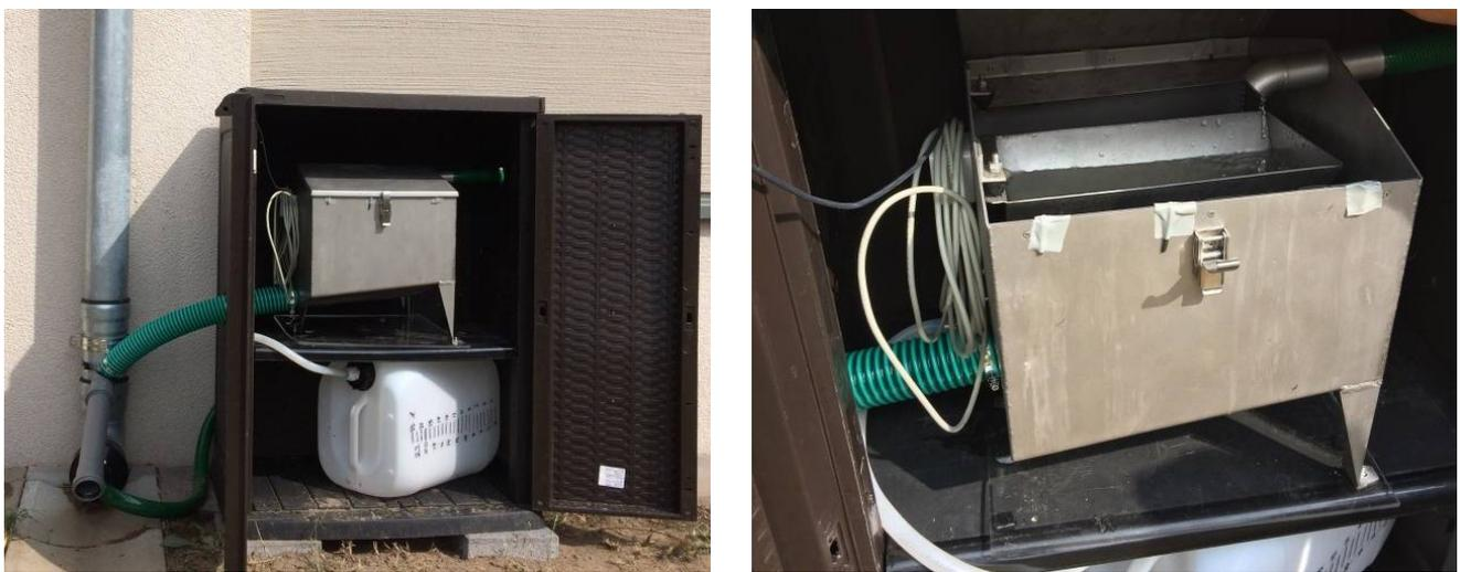
**Figure A3.** Tipping counter for measurement and sampling of roof runoff.
