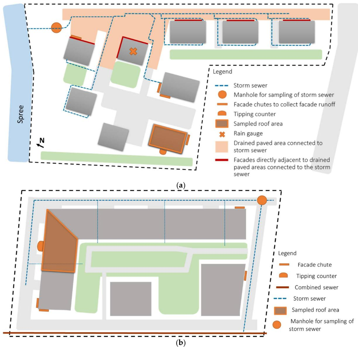
**Figure A1.** Schematic view of test site A (a) and test site B (b).
