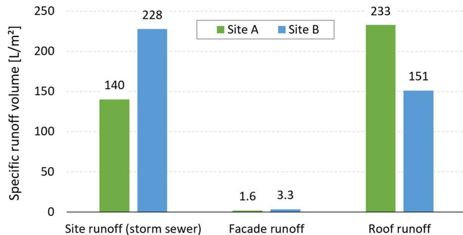
**Figure 1.** Specific runoff from surfaces drained to the storm sewer resulting from analysed storm events in test sites A and B.
