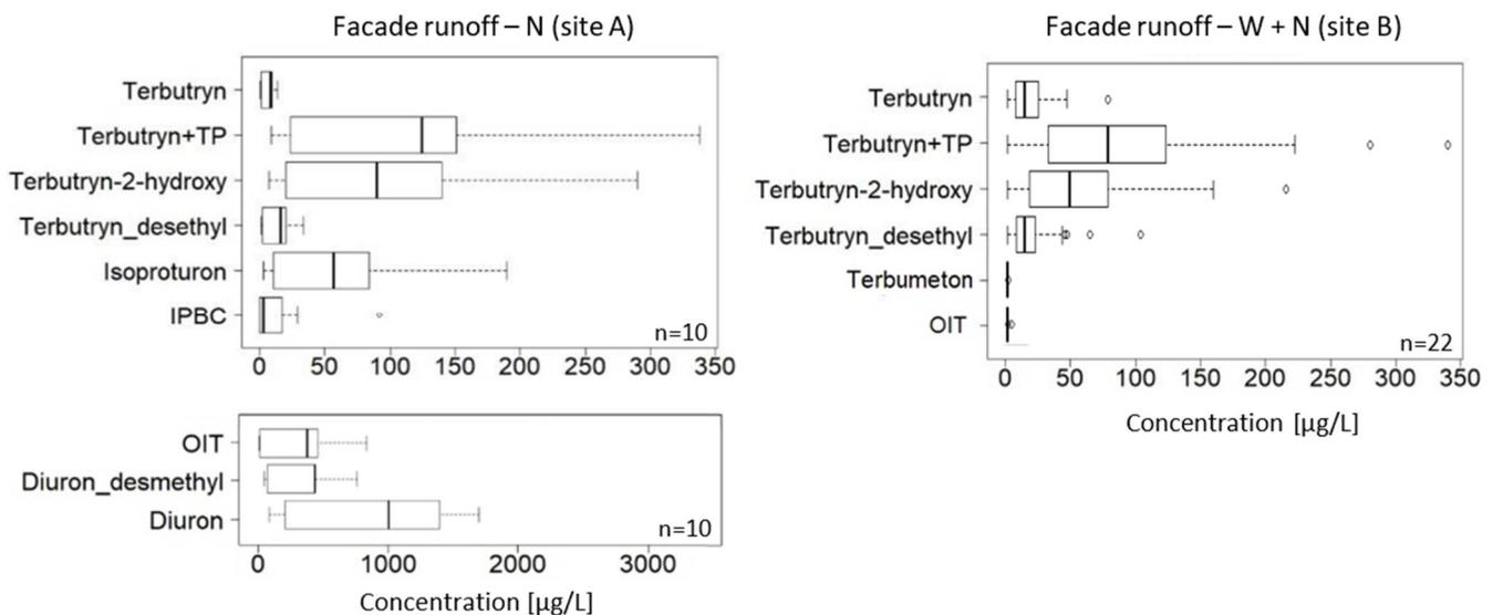
**Figure 2.** Concentration of biocides in façade runoff of painted façades at site A (north) and B (west and north).
