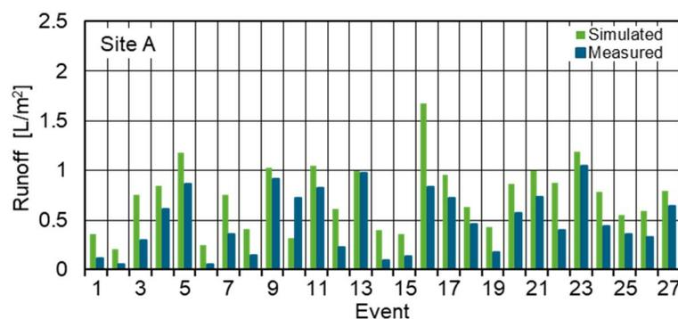
**Figure A8.** Measured and simulated façade runoff of buildings at test site A and site B for 27 and 26 events, respectively. Events with more than 10 mm rainfall were taken into account as a basis for the prediction.
