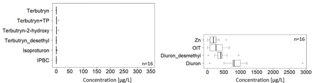
**Figure A7.** Concentrations of biocides in façade runoff from west façades at test site A.
