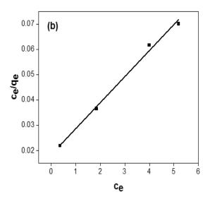
Figure 4. (a) Freundlich isotherm; (b) Langmuir isotherm for sorption of dyes using CPSMNPs.
