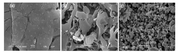
Figure 1. SEM image of (a) PS, (b) CPS, and (c) CPSMNPs.
