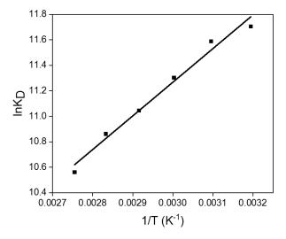
**Figure 6.** The plot of lnKD versus 1/T for estimation of thermodynamic parameters for MY sorption on CPSMNPs.
