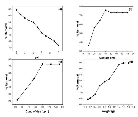
**Figure 3.** Effect of various parameters on the adsorption of MY using CPSMNPs: (a) effect of pH; (b) effect of contact time; (c) effect of initial concentration; (d) effect of adsorbent dose.
