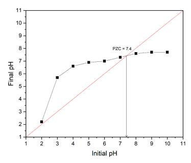
Figure 2. Point of zero charges of CPSMNPS adsorbent.
