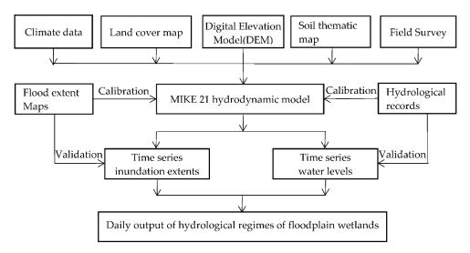
Figure 2. Flowchart of the calibration and validation process used to build the hydrodynamic model.
