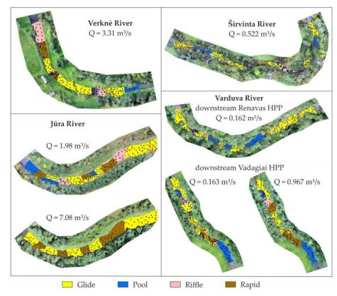
**Figure 5.** Distribution of the hydromorphological units and point measurements of hydraulic parameters across the selected case studies at certain discharges.
