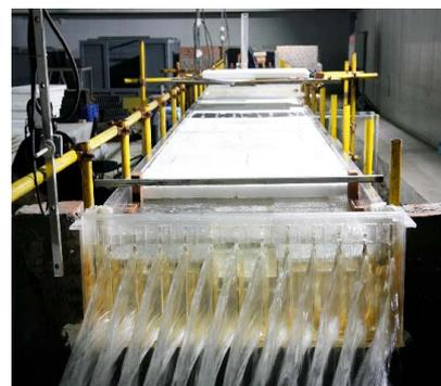
Figure 10. Experimental flume section with main channel and floodplain: (a) section topography showing ice cover, riverbed distribution, and cross-sectional relative-unit discharge; (b) photo of experimental flume.
