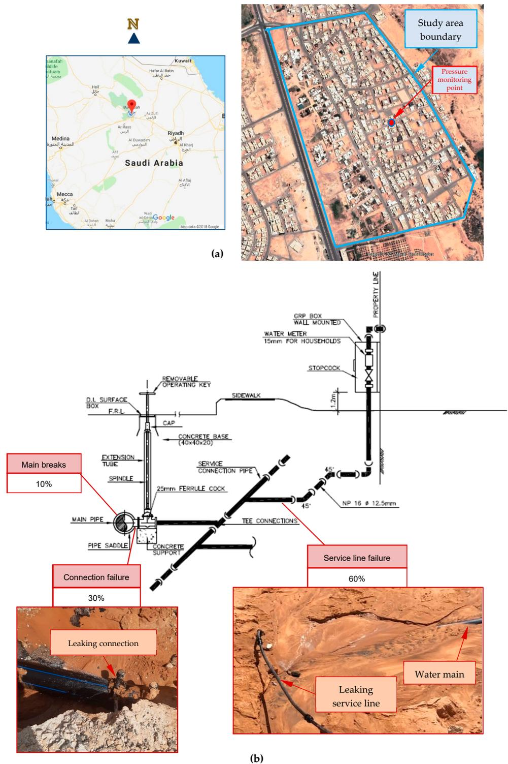
**Figure 1.** Study area and problem identification, (a) location of the study area the in Buraydah City of Qassim Region, (b) service connection details showing percentage contribution of each structural failure, 60% leaking service line, and 30% leaking connections.
