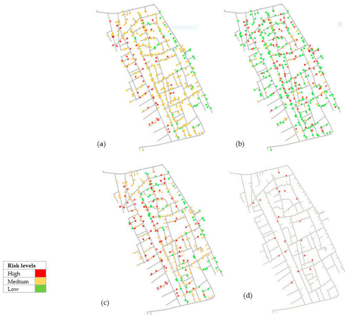
**Figure 9.** Spatial display of risk-based priority levels for service connections for inspection and rehabilitation of service connections, (a) consequence index, (b) vulnerability index, and (c) overall risk index, (d) model validation results, where all the 21 service connections repaired in response to customer complaints were ranked as high-risk connections by the developed model.
