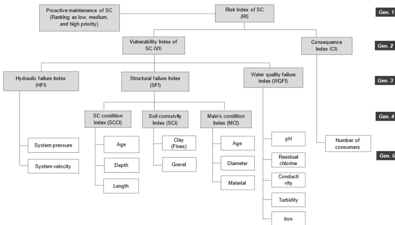
Figure 2. Risk-based methodology of the decision support system (DSS) for service connections' proactive maintenance planning.
