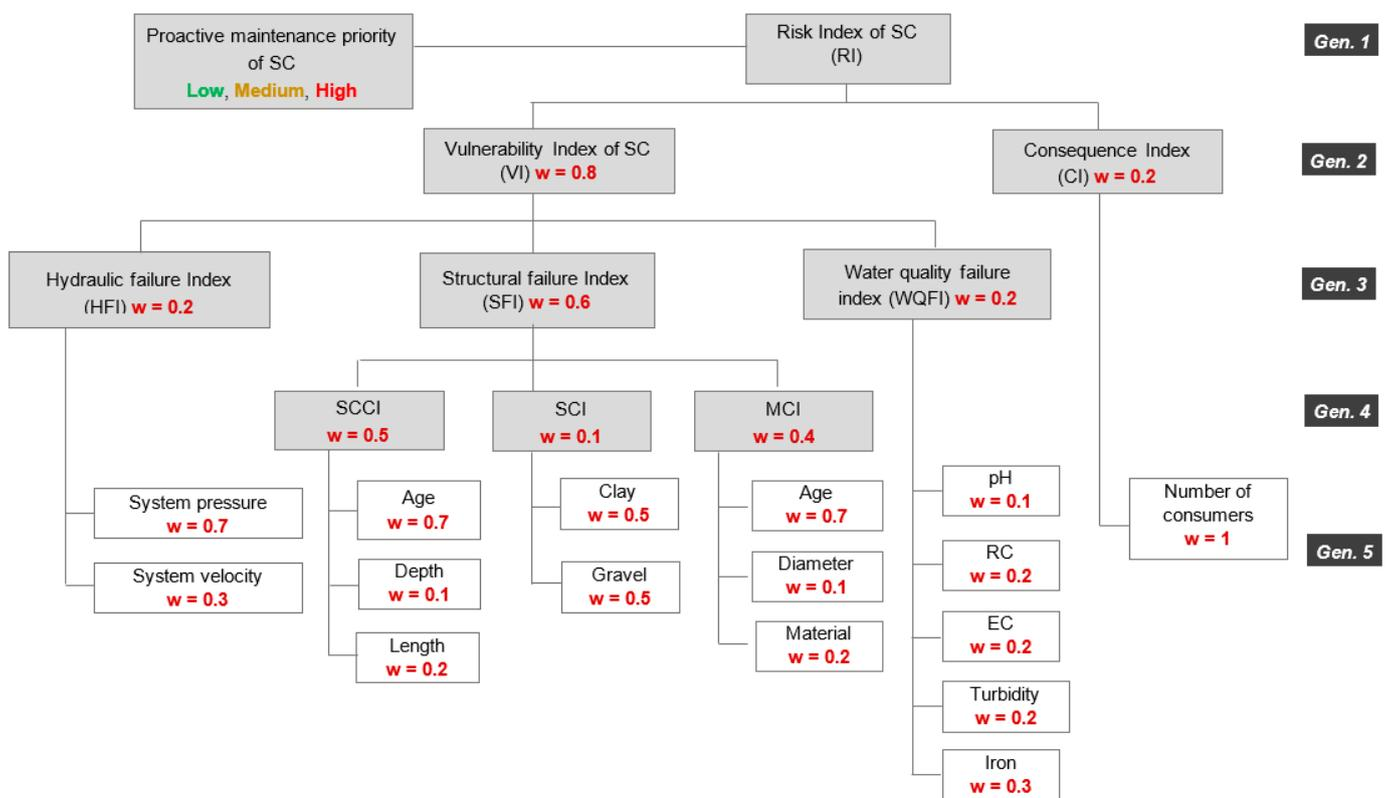
Figure 7. Weighting scheme by Fuzzy-AHP showing input data variables at Gen. 5, risk factors at Gen. 2 to Gen. 4, and risk index (RI) at the top.
