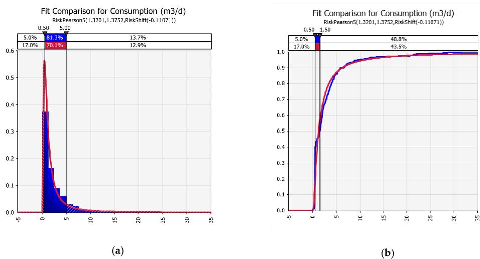
**Figure 5.** Water consumption in the study area, (a) probability density graph, (b) cumulative density graph (drawn using licensed version of @Risk Version 8 software). Horizontal axis shows water consumption ( $m^3/day$ ) and vertical axis represents probability values. Input data are shown in blue color and red line represents the Pearson 5 distribution.
