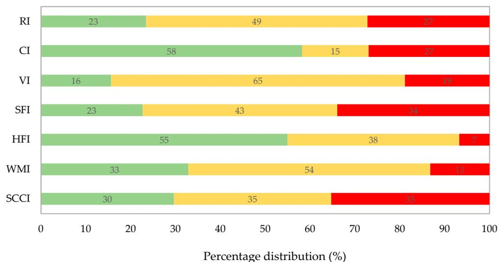
**Figure 8.** Summary of calculated indices. Risk index (RI), consequence index (CI), vulnerability index (VI), structural failure index (SFI), hydraulic failure index (HFI), water main condition index (WMI), and service connection condition index (SCCI).
