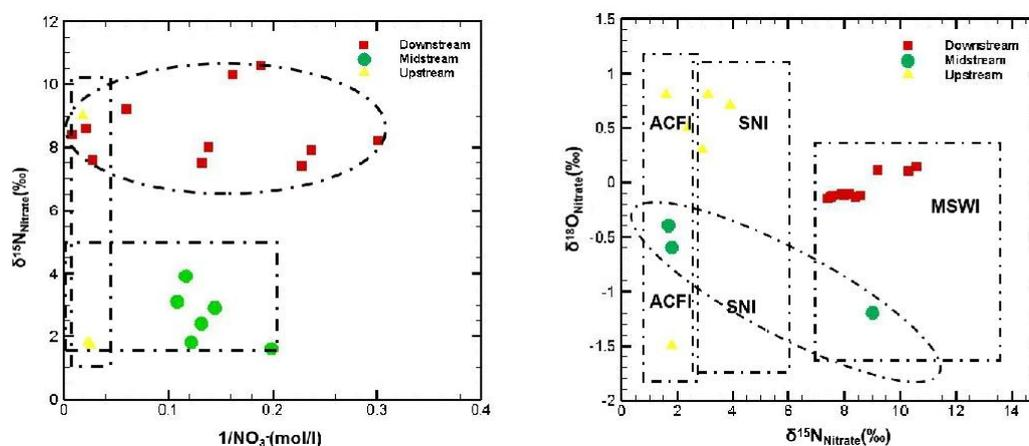
**Figure 2.** Keeling plot of  $1/NO_3^-$  and  $\delta^{15}N_{NO_3}$  (‰) and the relationship of  $\delta^{15}N_{Nitrate}$  (‰) and  $\delta^{18}O_{Nitrate}$  (‰) [4] in groundwater of the Yiluo River watershed during the dry season. MSWI represents manure and sewage waste input. SNI represents sediment nitrogen input. ACFI represents agricultural chemical fertilizer input.
