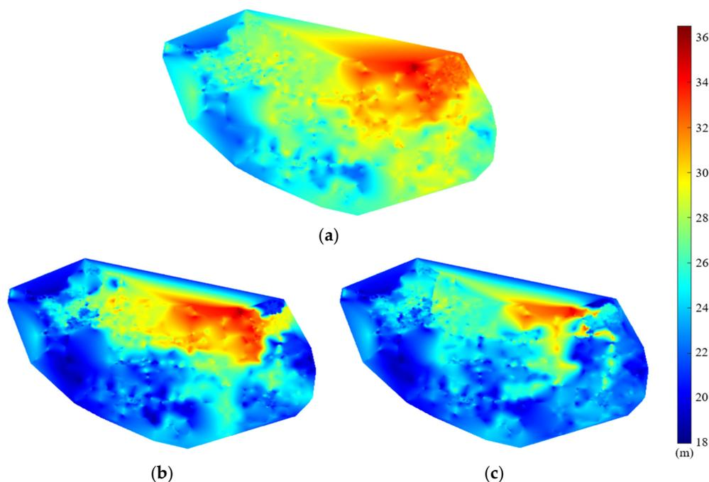
**Figure 8.** Pressure distribution in peak demand period: (a) Original; (b) Scheme A; (c) Scheme B.
