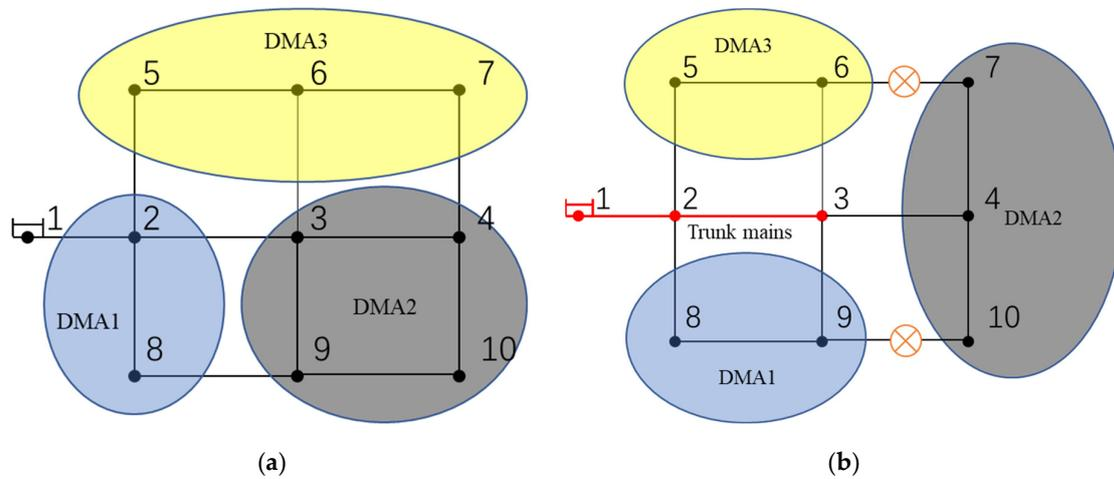
**Figure 1.** The Schematic diagrams of Schemes A and B: (a): Scheme A; (b): Scheme B.
