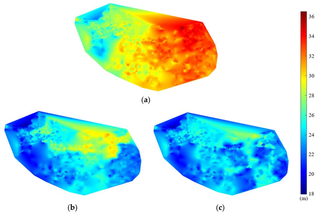
Figure 7. Pressure distribution in valley demand period: (a) Original; (b) Scheme A; (c) Scheme B.
