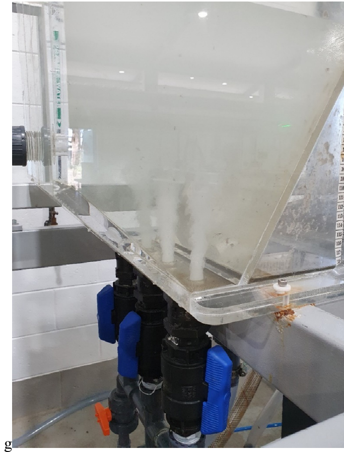
Figure S2. Generation of bubbles with tap water in pilot DAF contact zone.
