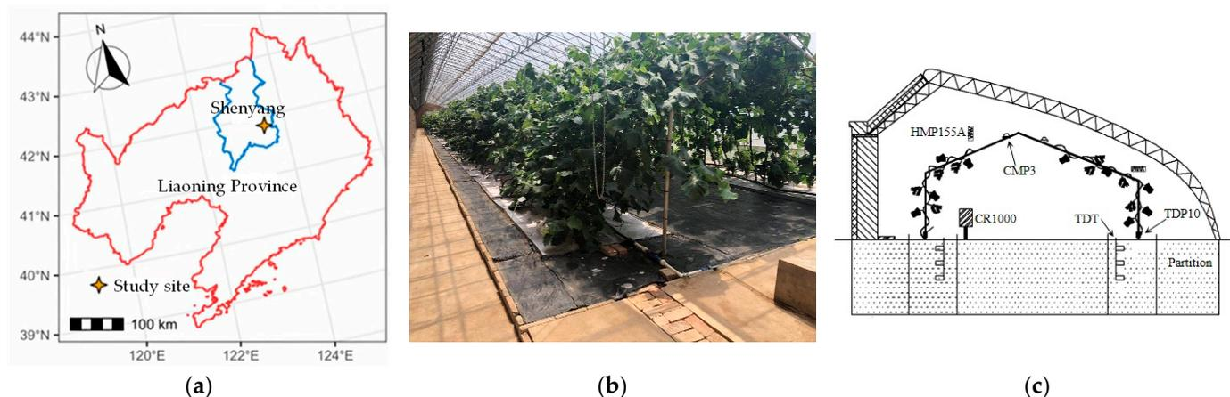
**Figure 1.** Experimental planting area of drip irrigation under plastic film and sensor layout. (a) Study site; (b) experimental planting area of drip irrigation under plastic film; (c) greenhouse structure and sensor layout.
