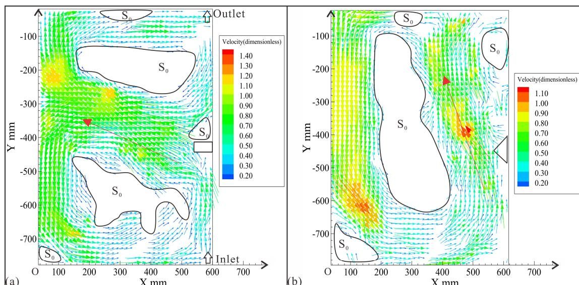
**Figure 2.** Distribution of the stagnant water area: (a) rectangular column,  $Q = 6.8 \text{ L/min}$ ,  $l = 0.44$ ; (b) triangular prism,  $Q = 6.8 \text{ L/min}$ ,  $l = 0.44$ .
