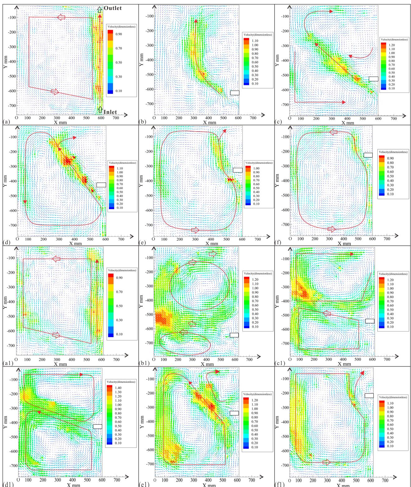
**Figure 4.** Vector distribution of the flow field under the influence of the rectangular column for  $Q = 3.7 \text{ L/min}$  and  $6.8 \text{ L/min}$ , respectively: (a–f) for  $3.7 \text{ L/min}$ ; (a1–f1) for  $6.8 \text{ L/min}$ . Vector distribution (a,a1) for no structure; (b,b1) for  $l = 0.19$ ; (c,c1) for  $l = 0.31$ ; (d,d1) for  $l = 0.44$ ; (e,e1) for  $l = 0.56$ ; (f,f1) for  $l = 0.69$ .
