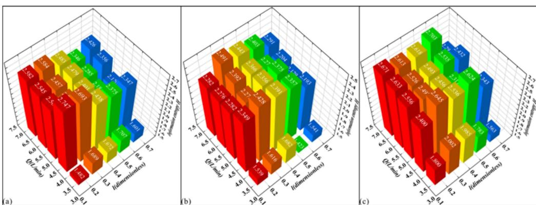
**Figure 12.** Calculation results of the information entropy of the two-dimensional flow field: (a) triangular prism; (b) semi-cylinder; (c) rectangular column.
