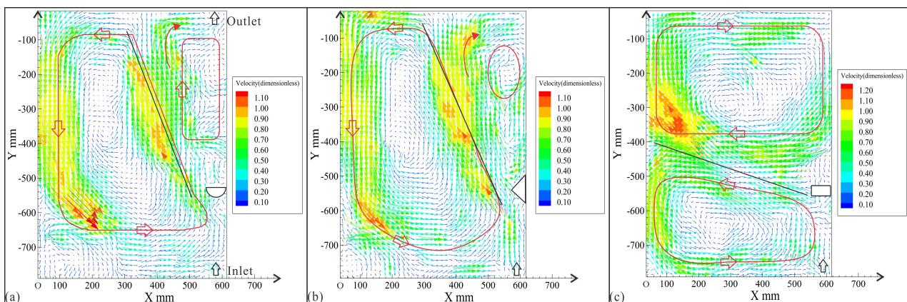
**Figure 7.** Straight line of the mainstream center (black line): (a) semi-cylinder,  $Q = 6.8 \text{ L/min}$ ,  $l = 0.31$ ; (b) triangular prism,  $Q = 6.8 \text{ L/min}$ ,  $l = 0.31$ ; (c) rectangular column,  $Q = 6.8 \text{ L/min}$ ,  $l = 0.31$ .
