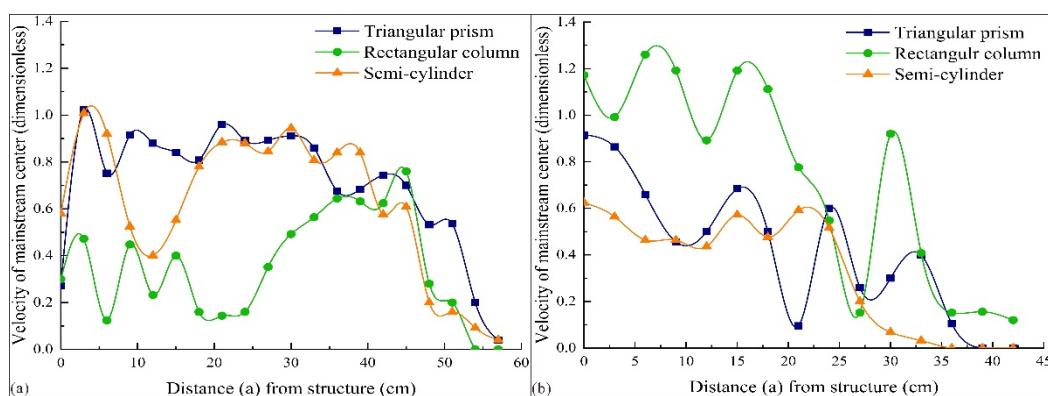
**Figure 8.** Variation in the velocity along the deflection mainstream center: (a)  $l = 0.31$ ; (b)  $l = 0.56$  ( $a$  is the straight-line distance from each point of the deflected mainstream to the structure).
