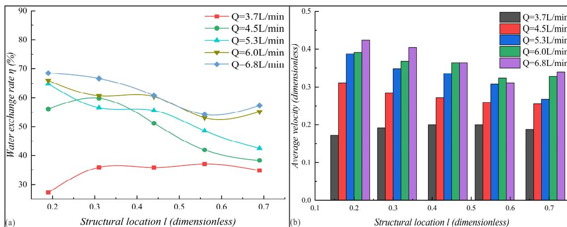
**Figure 9.** Calculation results for the triangular prism: (a) water exchange rate; (b) average velocity.
