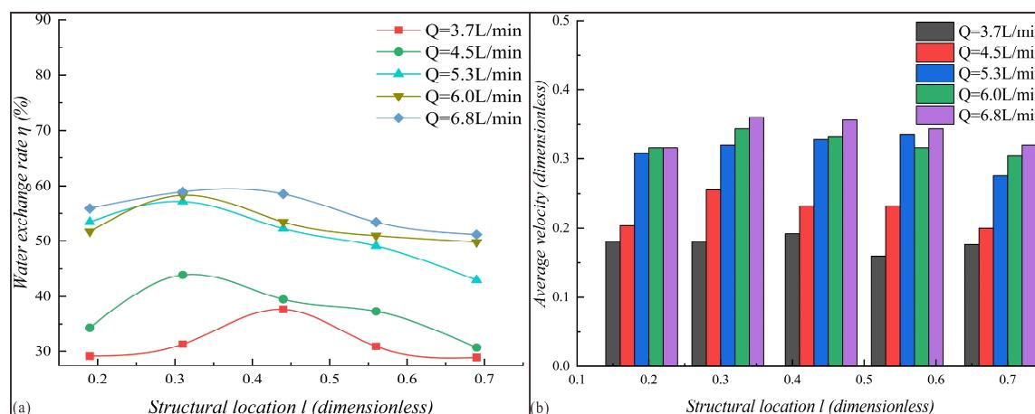
**Figure 10.** Calculation results for the semi-cylinder: (a) water exchange rate; (b) average velocity.
