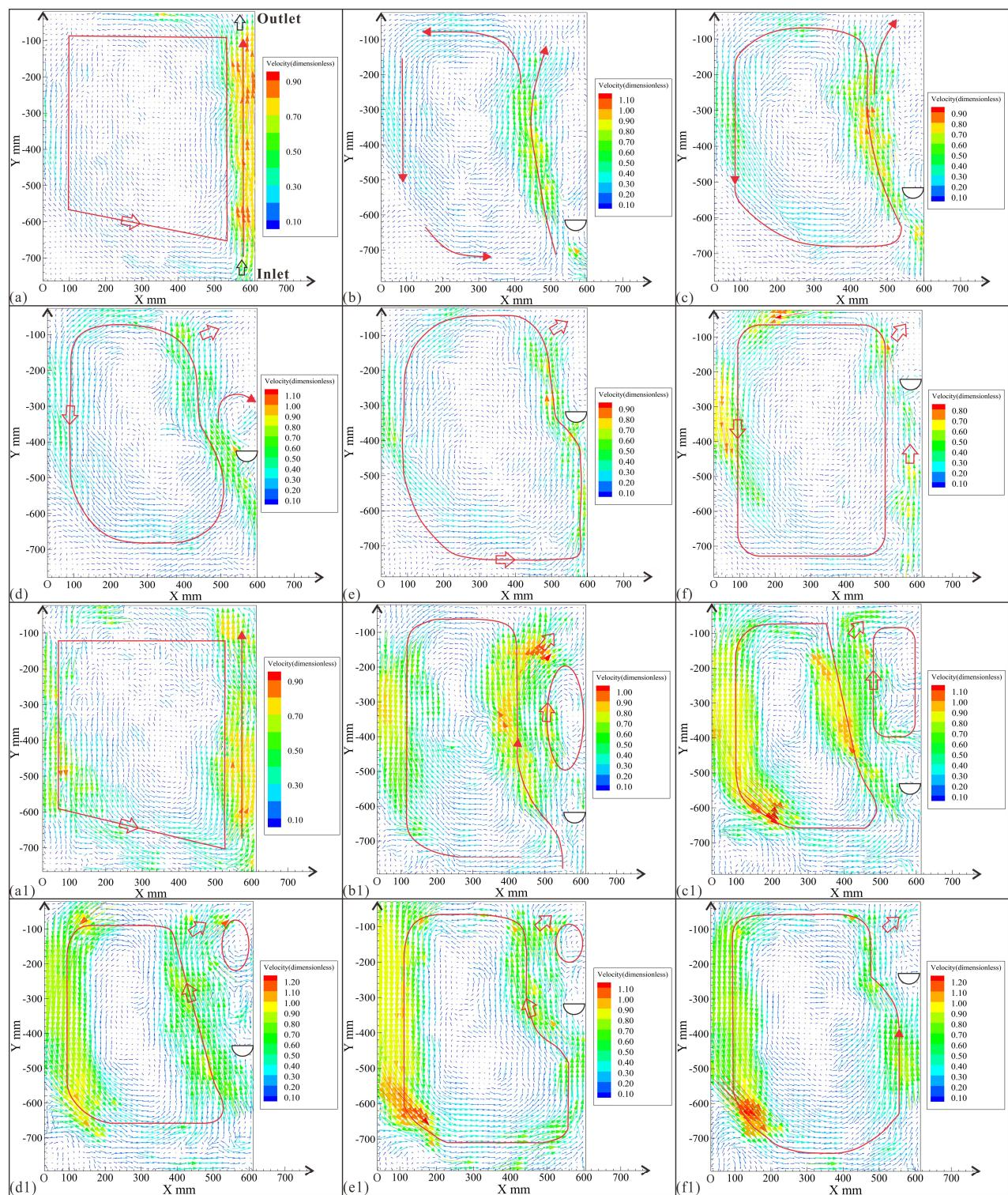
**Figure 6.** Vector distribution of the flow field under the influence of the semi-cylinder for  $Q = 3.7 \text{ L/min}$  and  $6.8 \text{ L/min}$ , respectively: (a–f) for  $3.7 \text{ L/min}$ ; (a1–f1) for  $6.8 \text{ L/min}$ . Vector distribution (a,a1) for no structure; (b,b1) for  $l = 0.19$ ; (c,c1) for  $l = 0.31$ ; (d,d1) for  $l = 0.44$ ; (e,e1) for  $l = 0.56$ ; (f,f1) for  $l = 0.69$ .
