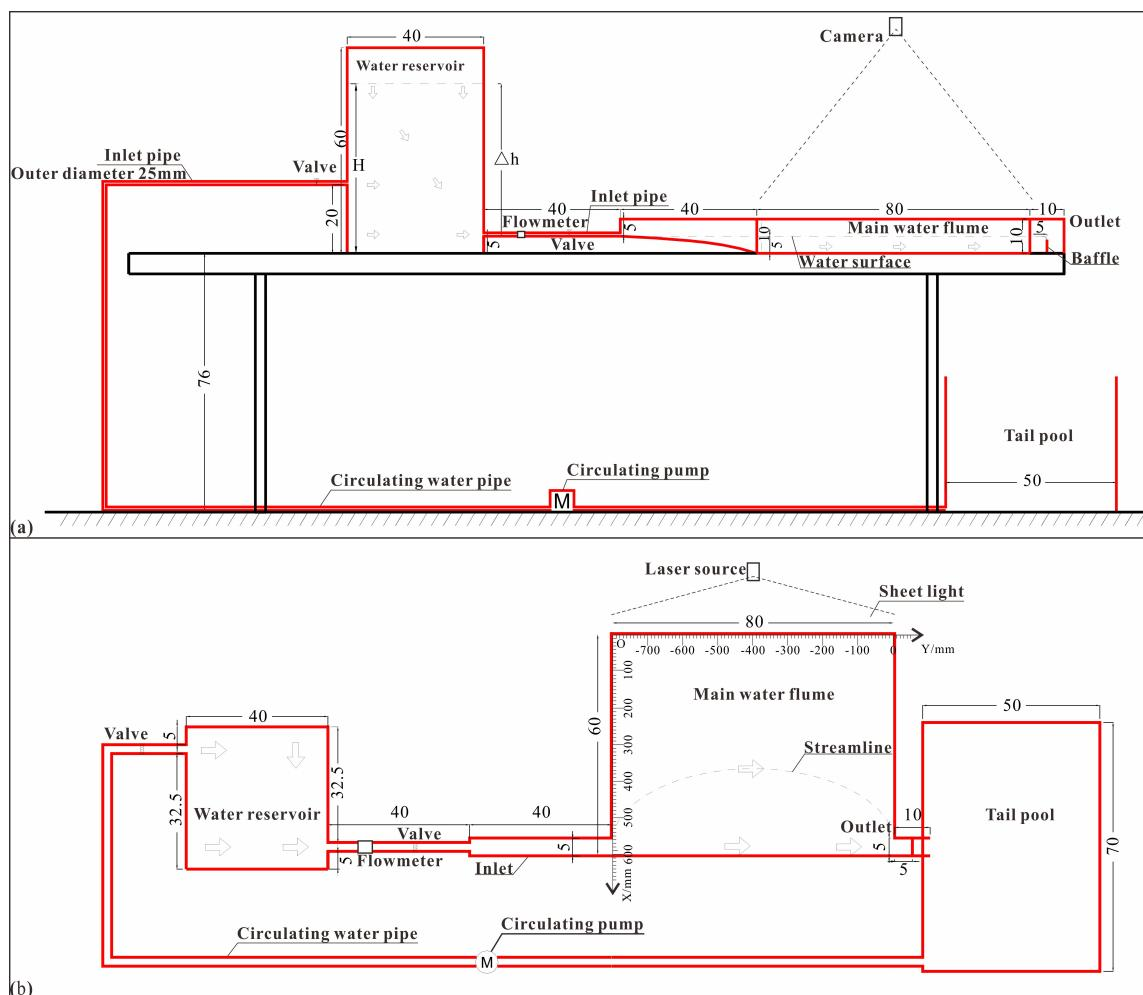
**Figure 1.** Experimental installation: (a) side view of the flume; (b) top view of the flume (point O is the axis origin, and the unit of the numbers in the figure is cm, except for those already indicated).
