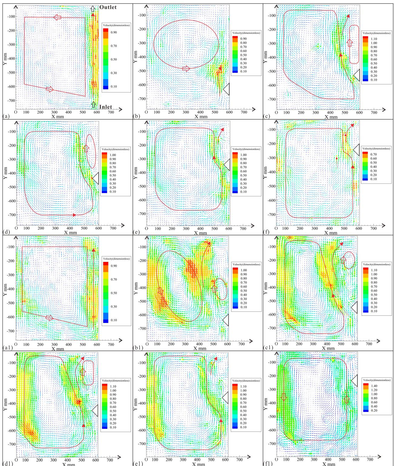
**Figure 5.** Vector distribution of the flow field under the influence of the triangular prism for  $Q = 3.7 \text{ L/min}$  and  $6.8 \text{ L/min}$ , respectively: (a–f) for  $3.7 \text{ L/min}$ ; (a1–f1) for  $6.8 \text{ L/min}$ . Vector distribution (a,a1) for no structure; (b,b1) for  $l = 0.19$ ; (c,c1) for  $l = 0.31$ ; (d,d1) for  $l = 0.44$ ; (e,e1) for  $l = 0.56$ ; (f,f1) for  $l = 0.69$ .
