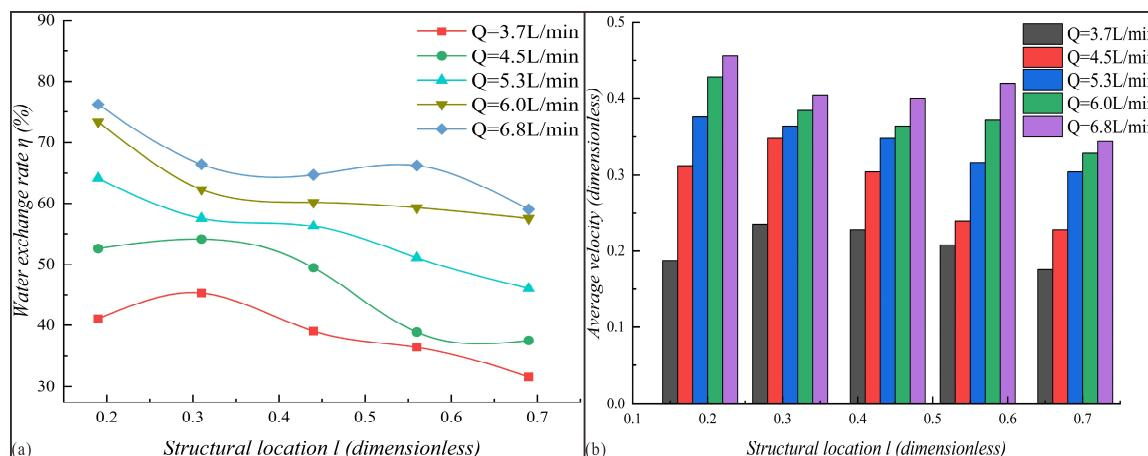
**Figure 11.** Calculation results for the rectangular column: (a) water exchange rate; (b) average velocity.
