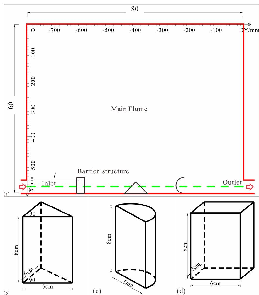
**Figure 3.** Schematic diagram of barrier structures in water body: (a) structure location; (b) triangular prism; (c) semi-cylinder; (d) rectangular column.
