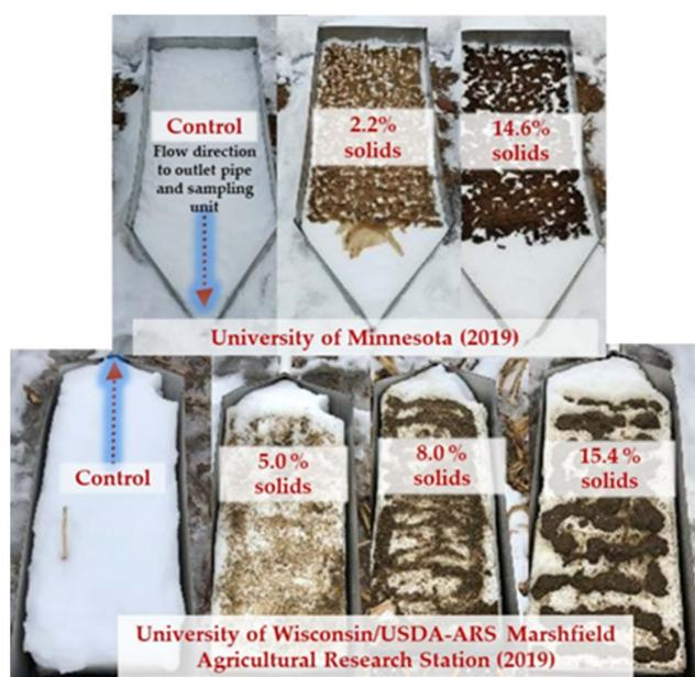
**Figure 1.** Photographs showing snowmelt runoff plots after manure application for the University of Minnesota and Marshfield Station (2019).
