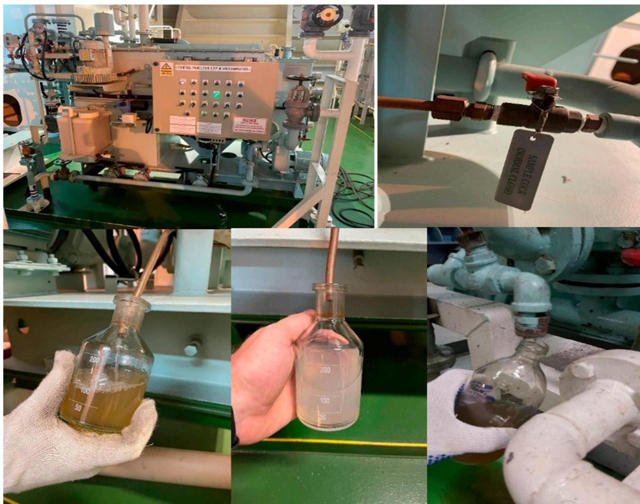
**Figure 1.** Ship “grey water” sampling from the transport vessel.
