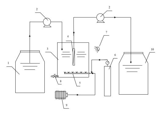
**Figure 1.** A schematic diagram of the pilot-scale MPBR system. (1)-Primary tank; (2)-peristaltic pumps, (3)-MPBR vessel, (4)-MBR membrane, (5)-air distributor, (6)-CO<sub>2</sub> gas cylinder, (7)-LED lamps, (8)-discharge valve, (9)-Air compressor, (10)-Discharge collector.
