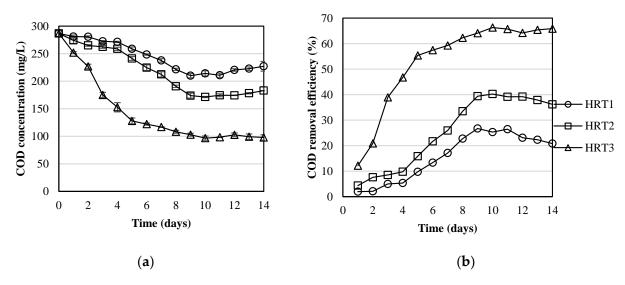
**Figure 5.** The change of (**a**) COD concentration and (**b**) COD removal efficiency in 2-fold diluted piggery wastewater over 14 days in *Chlorella vulgaris*-based MPBR at various hydraulic retention times (HRT1 = 1.25 days, HRT2 = 2.5 days, HRT 3 = 5 days).
