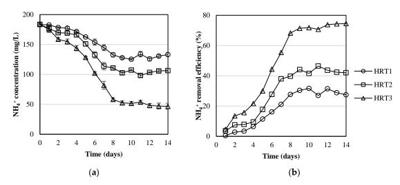
**Figure 3.** The change of (a)  $NH_4^+$  concentration and (b)  $NH_4^+$  removal efficiency in 2-fold diluted piggery wastewater over 14 days in *Chlorella vulgaris*-based MPBR at various hydraulic retention times (HRT1 = 1.25 days, HRT2 = 2.5 days, HRT 3 = 5 days).
