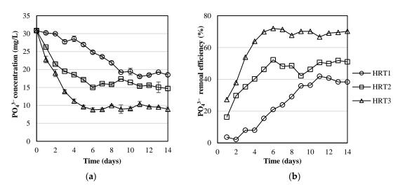
**Figure 4.** The change of (**a**)  $PO_4^{3-}$  concentration and (**b**)  $PO_4^{3-}$  removal efficiency in 2-fold diluted piggery wastewater over 14 days in *Chlorella vulgaris*-based MPBR at various hydraulic retention times (HRT1 = 1.25 days, HRT2 = 2.5 days, HRT 3 = 5 days).
