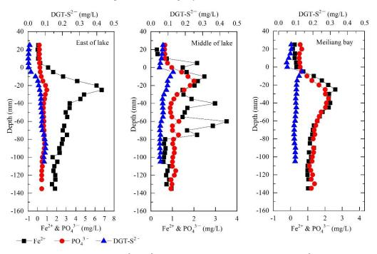
**Figure 5.** Concentrations of  $PO_4^{3-}$ ,  $Fe^{2+}$  in the profile of pore water and DGT-S<sup>2-</sup> in the profile of sediment of Taihu Lake.
