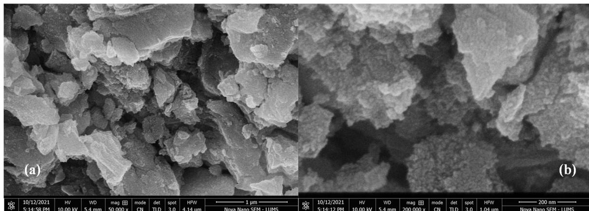
**Figure 4.** SEM micrographs of Fe NPs at 1  $\mu\text{m}$  (a), 200 nm (b).
