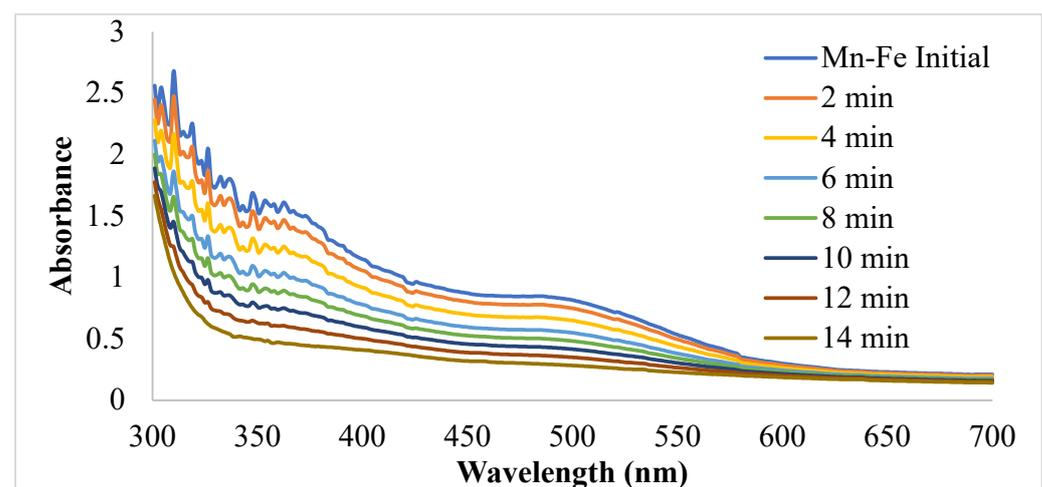
Figure 12. UV-visible spectra for photocatalytic degradation of CR using Fe-Mn NPs.
