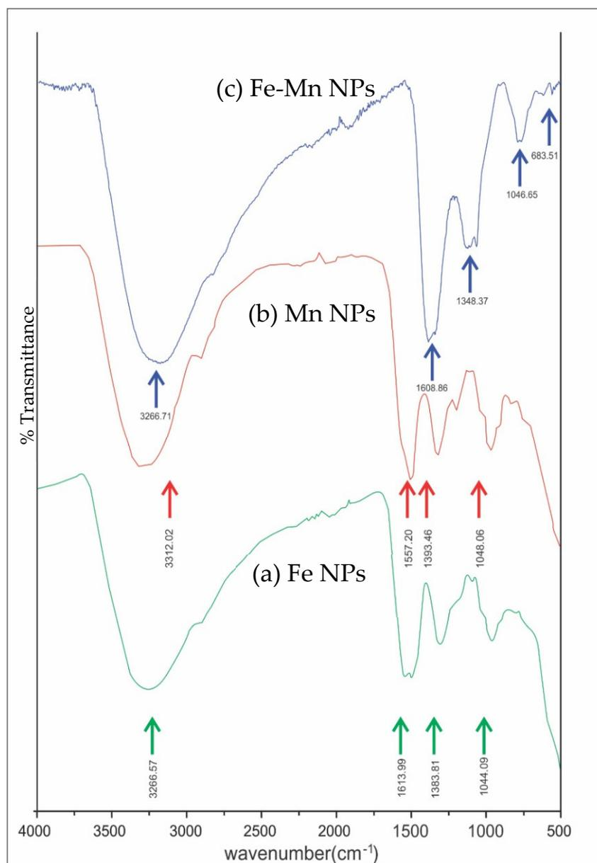
**Figure 2.** FTIR spectra of (a) Fe NPs, (b) Mn NPs (c) Fe-Mn NPs.
