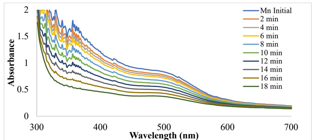
Figure 11. UV-visible spectra for photocatalytic degradation of CR using Mn NPs.
