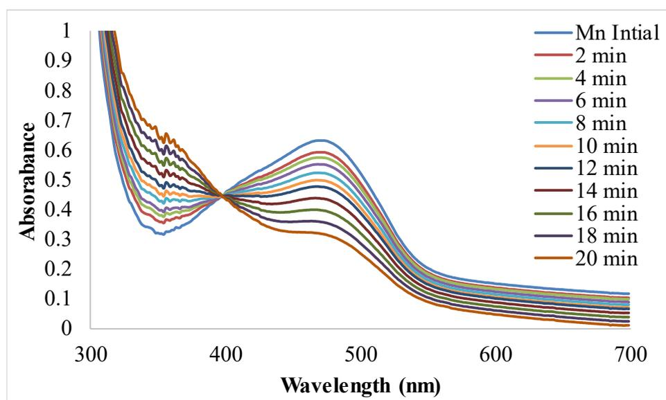
**Figure 8.** UV-visible spectra for photocatalytic degradation of MO using Mn NPs.
