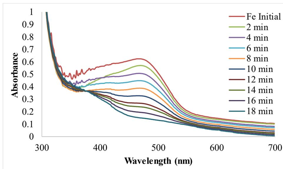
**Figure 7.** UV-visible spectra for photocatalytic degradation of MO using Fe NPs.
