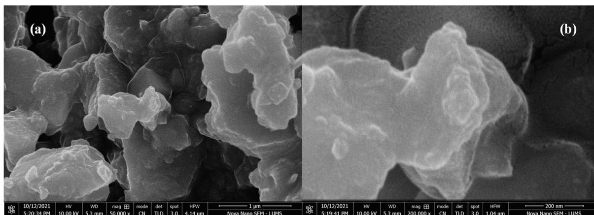
**Figure 5.** SEM micrographs of Mn NPs at 1  $\mu\text{m}$  (a), 200 nm (b).
