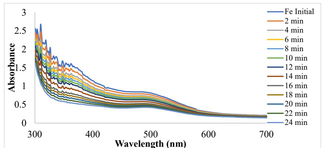
**Figure 10.** UV-visible spectra for photocatalytic degradation of CR using Fe NPs.
