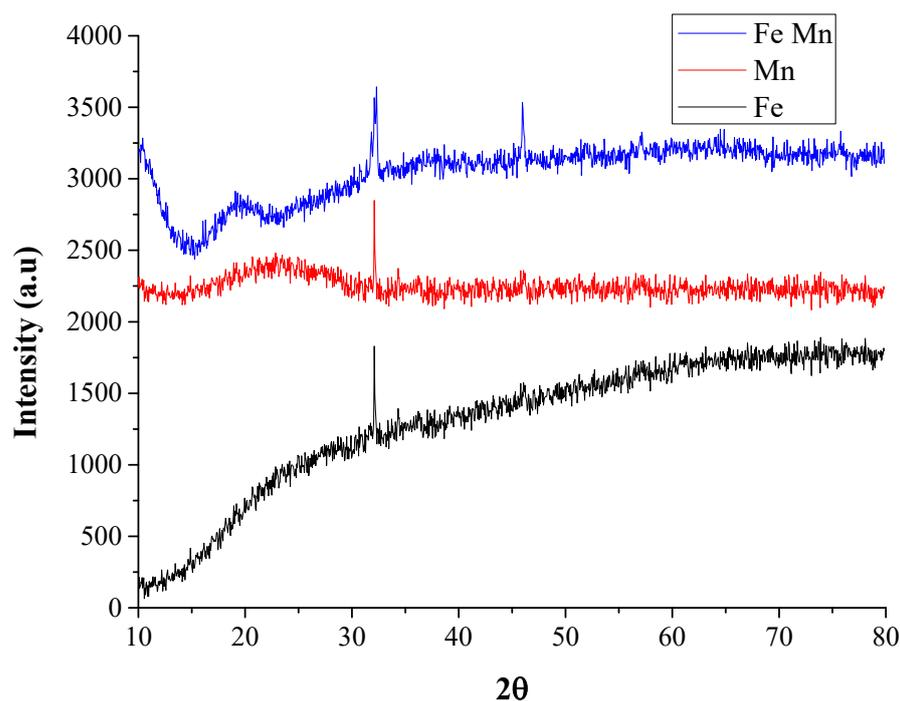
Figure 3. XRD spectra Fe, Mn and Fe-Mn NPs.
