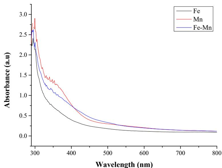
**Figure 1.** UV-visible spectra of Fe, Mn and Fe-Mn NPs.
