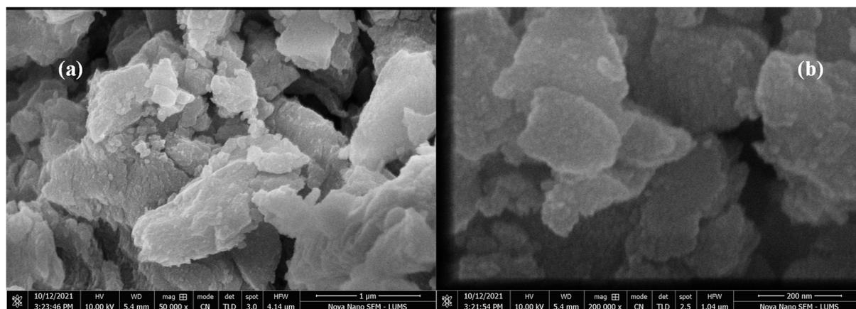
**Figure 6.** SEM micrographs of Fe/Mn NPs at 1  $\mu\text{m}$  (a), 200 nm (b).
