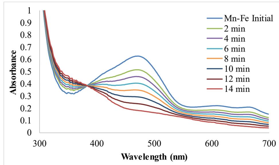
**Figure 9.** UV-visible spectra for photocatalytic degradation of MO using Fe-Mn NPs.
