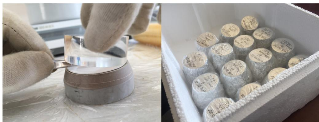
**Figure 6.** Insertion of filter paper and protection of samples from evaporation.
