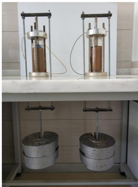
**Figure 4.** Preparation of reconstituted samples by consolidation from slurries.
