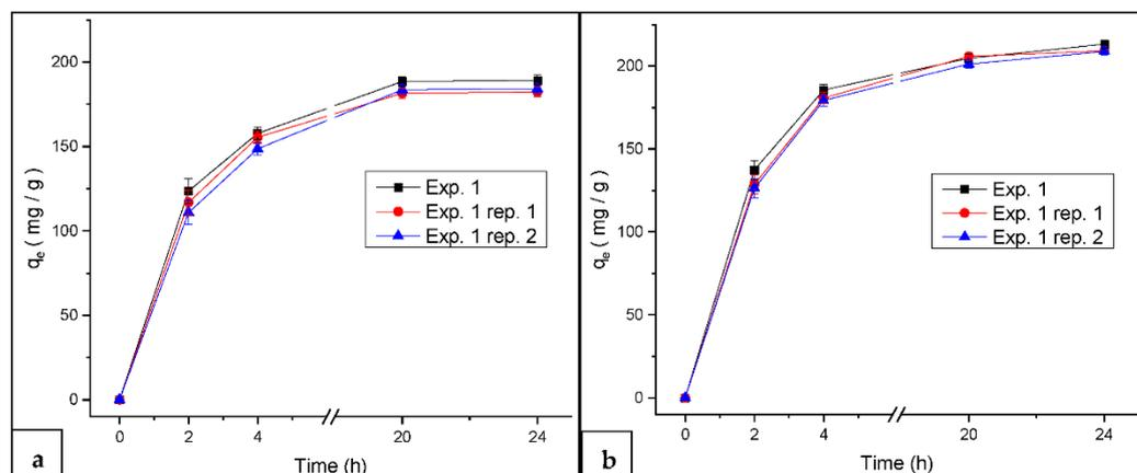
**Figure 4.** MB adsorption as a function of time at pH 6.0 and 37.5 °C using (a) SAP and (b) SAP-AC as adsorbents.
