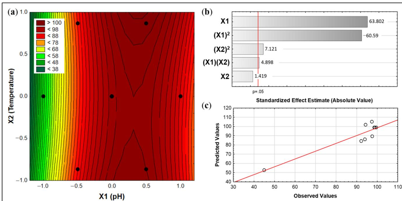
**Figure 10.** Response surface for the percent adsorption removal of MB by SAP-AC after 24 h of continuous recirculation. (a) Contour plot of adsorption as a function of pH and temperature; (b) Pareto chart of standardized effect estimates; and (c) residual plot showing observed vs. predicted values. ( $C_{MB,0} = 50$  ppm;  $V = 300$  mL;  $m_{SAP-AC,0} = 70$  mg.).
