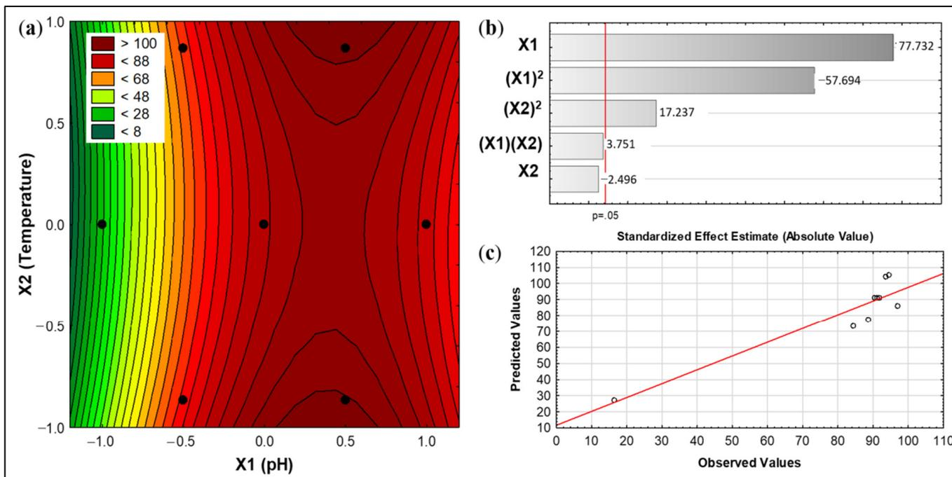
**Figure 9.** Response surface for the percent adsorption removal of MB by SAP after 24 h of continuous recirculation. (a) Contour plot of adsorption as a function of pH and temperature; (b) Pareto chart of standardized effect estimates; and (c) residual plot showing observed vs. predicted values. ( $C_{MB,0} = 50$  ppm;  $V = 300$  mL;  $m_{SAP,0} = 70$  mg.).
