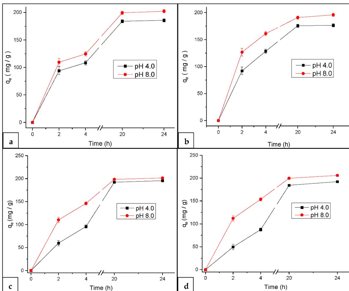
**Figure 6.** MB adsorption as a function of time at (a) 25 °C and (b) 50 °C using SAP and at (c) 25 °C and (d) 50 °C using SAP-AC as adsorbent.
