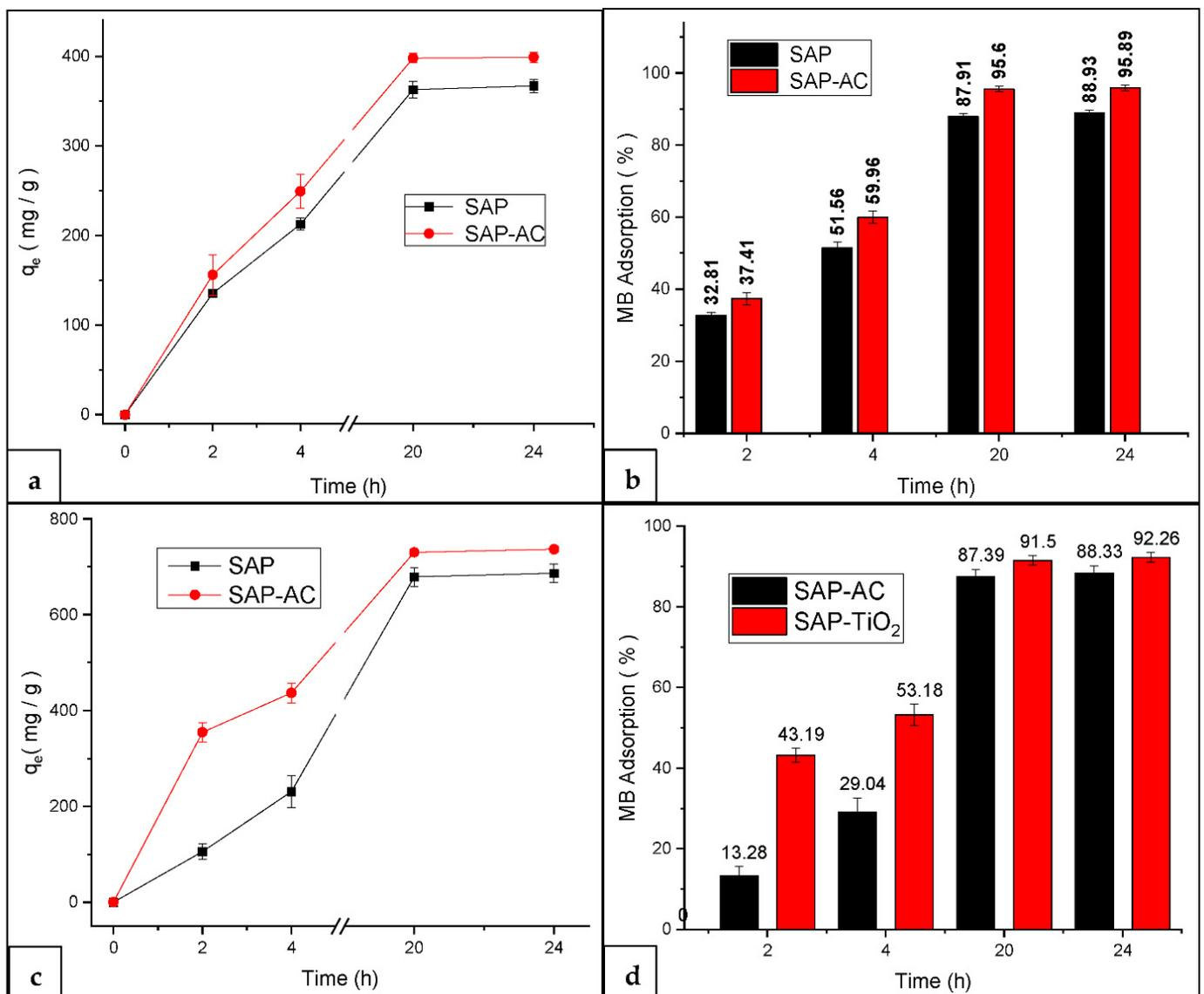
**Figure 11.** MB adsorption as a function of time. (a) Adsorption capacity and (b) percent adsorption using 100 ppm, and (c) adsorption capacity and (d) percent adsorption using 200 ppm initial concentration.
