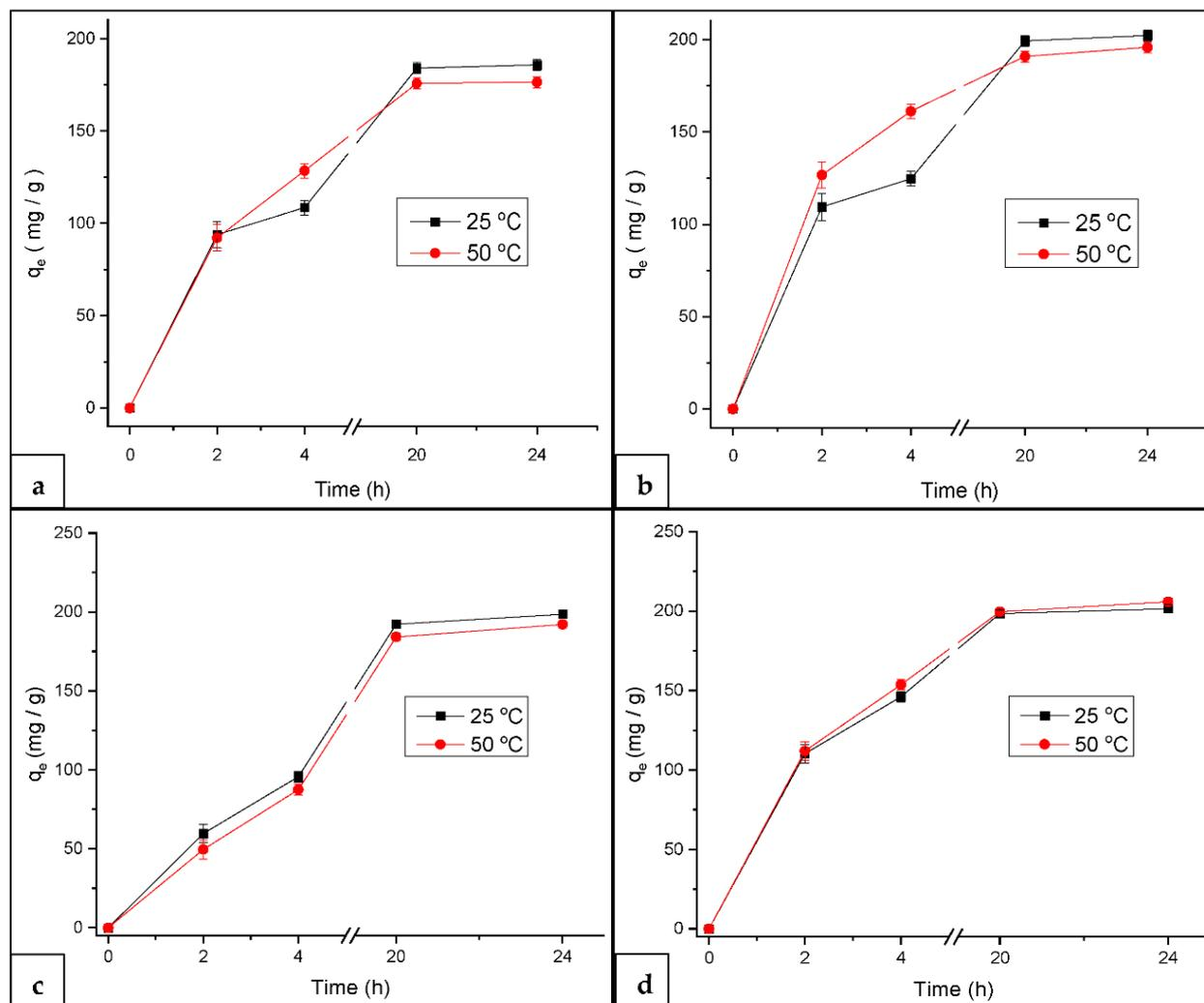
**Figure 7.** MB adsorption capacity as a function of time at (a) pH 4.0 and (b) pH 8.0 using SAP and at (c) pH 4.0 and (d) pH 8.0 using SAP-AC as adsorbent.
