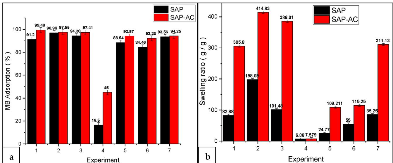
**Figure 8.** Comparison of various reaction parameters using SAP and SAP-AC for (a) percent MB adsorption and (b) swelling ratio.
