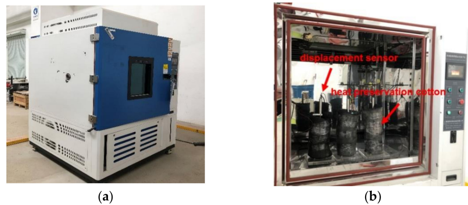
Figure 3. Test site layout: (a) Multifunctional physical simulation test platform (b) Soil column ready for test.
