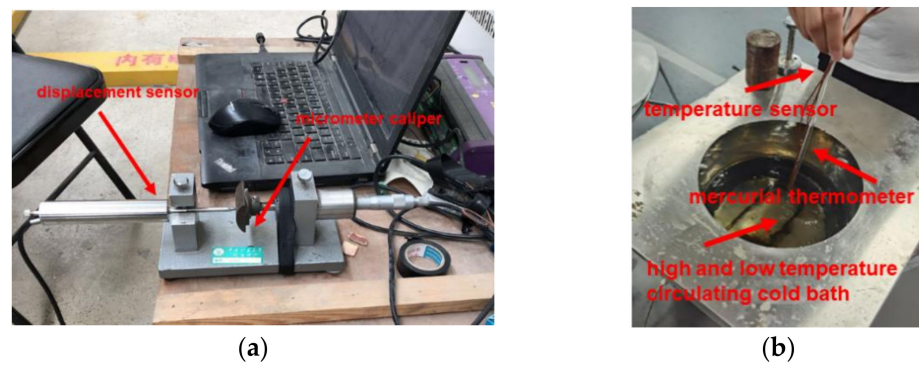
Figure 5. Sensor calibration: (a) Calibration of displacement sensor with screw micrometer (b) Temperature sensor calibration.
