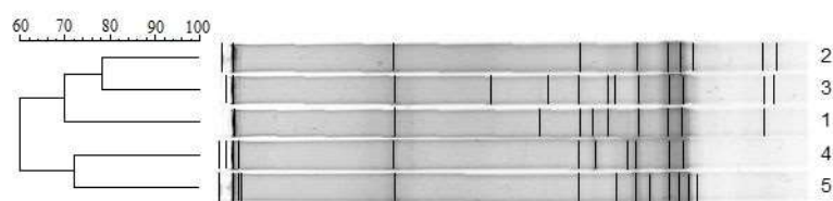
Figure 7. Electrophoretic profiles of denaturing gradient gel (DGGE). Sample 1 is the sludge used at the start (inoculation). Sample 2 is the sludge collected during the steady state of Phase I. Sample 3 is the sludge collected during the steady state of Phase II. Sample 4 is the sludge collected during the steady state of Phase III. Sample 5 is the sludge collected during the steady state of Phase IV.
