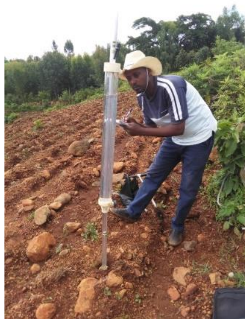
Figure 3. Field measurements of infiltration rate using a Guelph permeameter.
