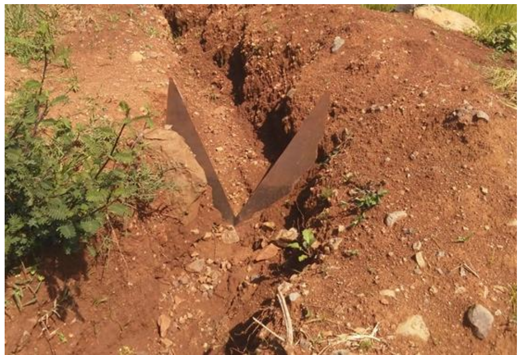
Figure 2. A typical triangular V-notch weir installed on the infiltration furrows at upslope positions of the Debre Mawi watershed.
