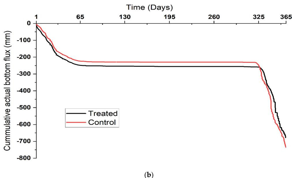
**Figure 3.** Soil water storage under treated versus control cultivated land on gentle slope (a), Cumulative bottom flux under treated versus control cultivated land on gentle slope (b).
