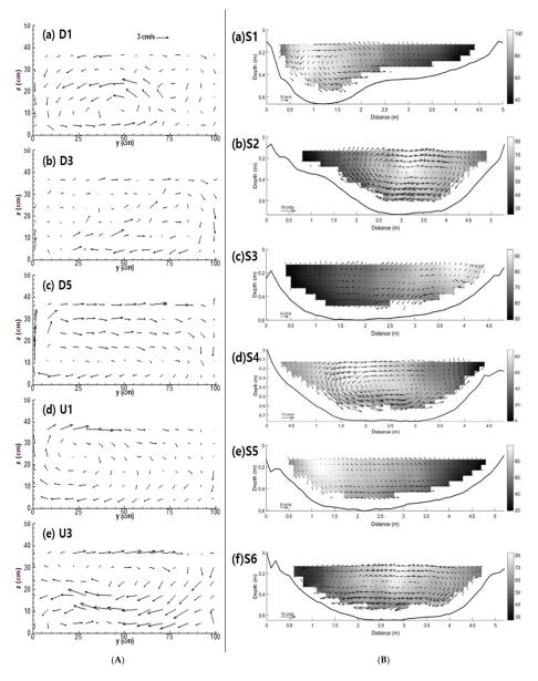
**Figure 6.** (A) Secondary flow patterns at representative cross-sections for case 402 in laboratory meandering channel (y denotes lateral coordinate from left to right bank, and z denotes vertical coordinate from bottom to water surface). (B) Secondary flow patterns at each cross-section of AMC 315 in nature-like channel.
