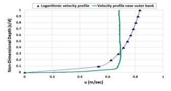
**Figure 1.** Comparison of vertical distribution for longitudinal flow velocity in straight and curved channels (adapted from Mozaffari et al. [28]).
