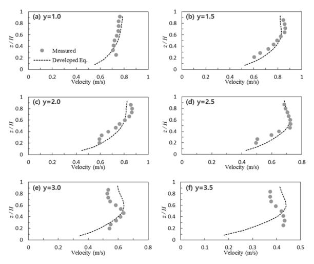
**Figure 7.** Comparison between measured velocity (dot) and that estimated by Equation (7) (line) at Section S4 of AMC 315 in nature-like channel (y denotes lateral coordinate from left to right bank).
