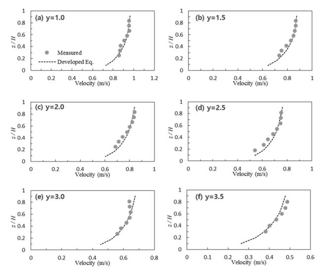
**Figure 8.** Comparison between measured velocity (dot) and that estimated by Equation (7) (line) at Section **S5** of AMC 315 in nature-like channel.
