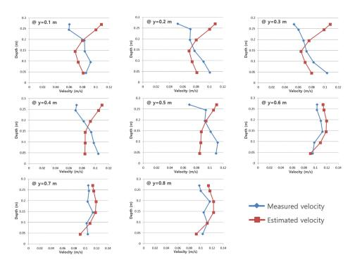
**Figure 5.** Comparison between measured velocity (blue line) and that estimated by Equation (7) (red line) in laboratory meandering channel at Section U1 (y denotes lateral coordinate from left to right bank).
