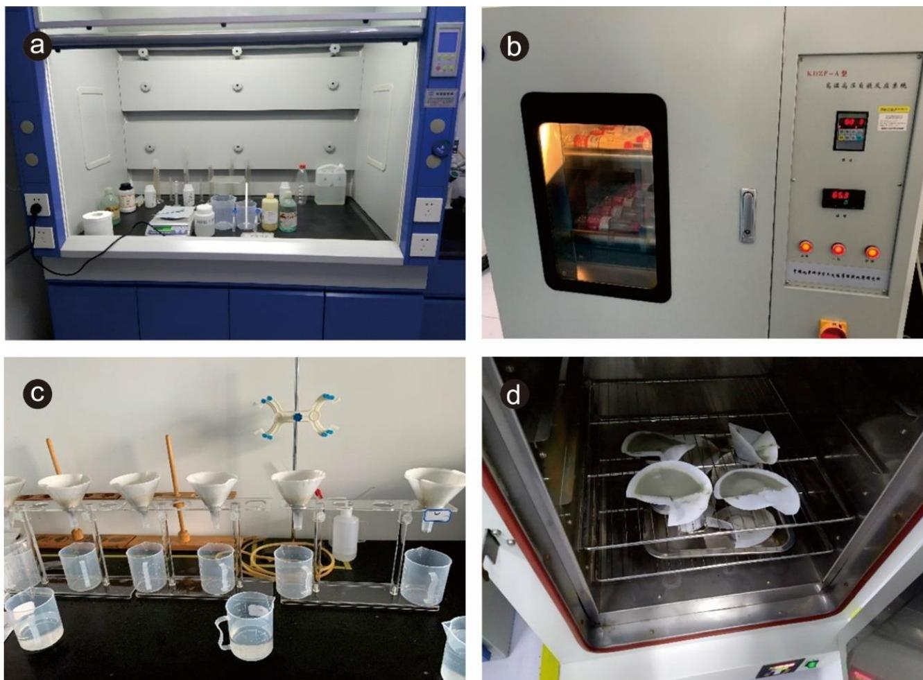
**Figure 3.** Experimental design and procedures. (a) The fume cupboard treatment of acid-added samples; (b) samples in the automatic rotary reactor system; (c) sample precipitation filtration; (d) precipitation placed in incubator for drying.
