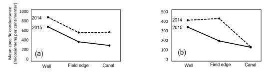
**Figure 3.** Mean specific conductance values (**a**) and bicarbonate concentrations (**b**) measured at 3 wells, risers, and associated canal in 2014 and one well, riser, and associated canal in 2015.
