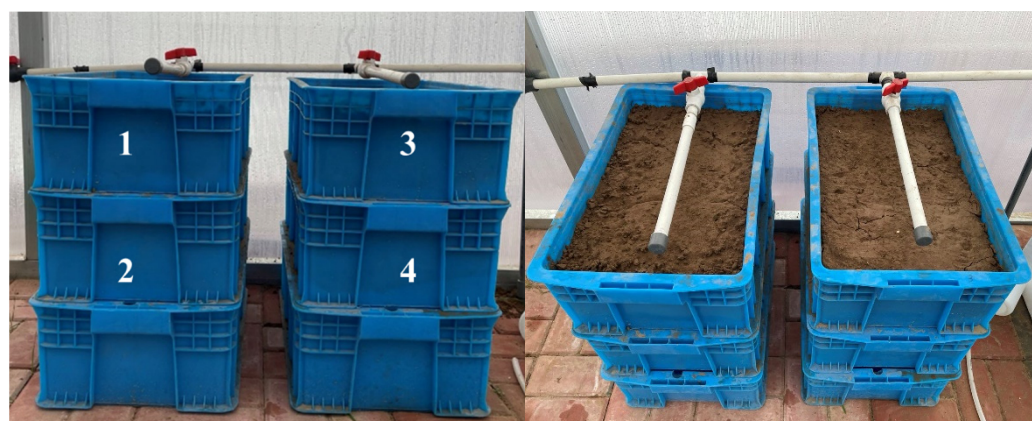
Figure 2. Photos of multistage soil box percolation system.
