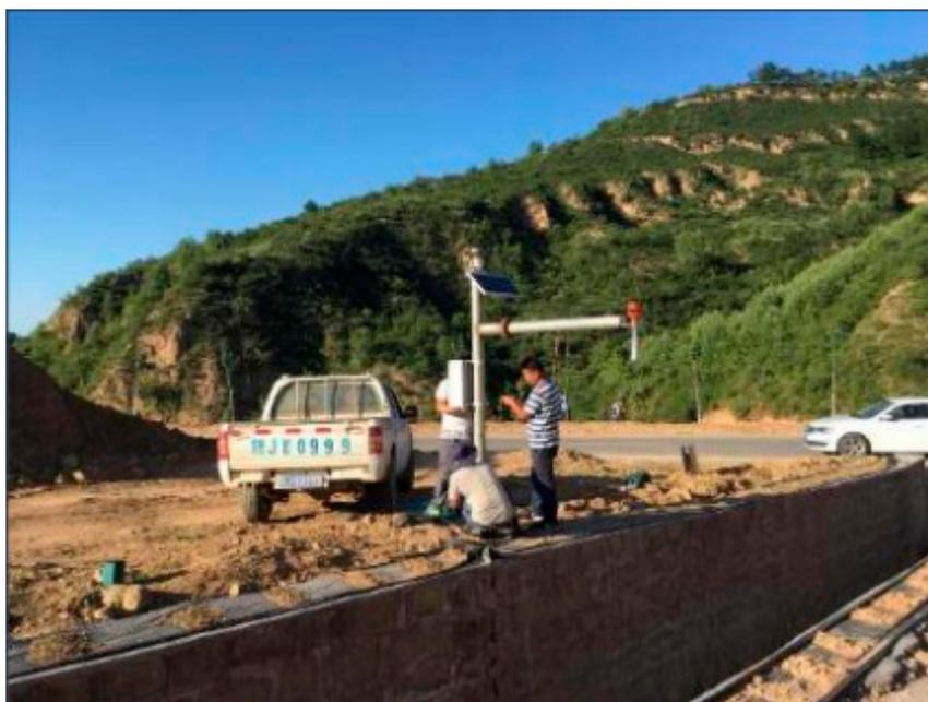
Figure 4. The auto-recording tipping bucket rain gauge and radar water level sensor at watershed outlet.
