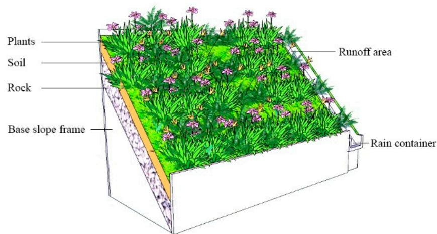
**Figure 2.** Structural diagram of the slope system.
