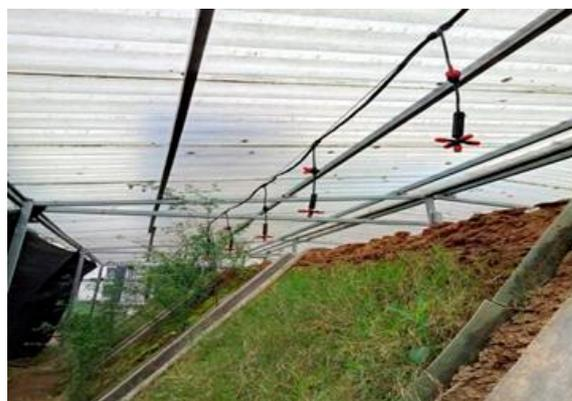
Figure 1. Experimentally simulated slope.
