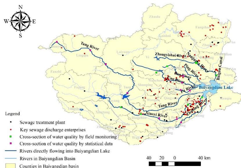
**Figure 2.** Cross-section of the water quality monitoring and key monitoring point sources of wastewater discharge in the Baiyangdian Basin.
