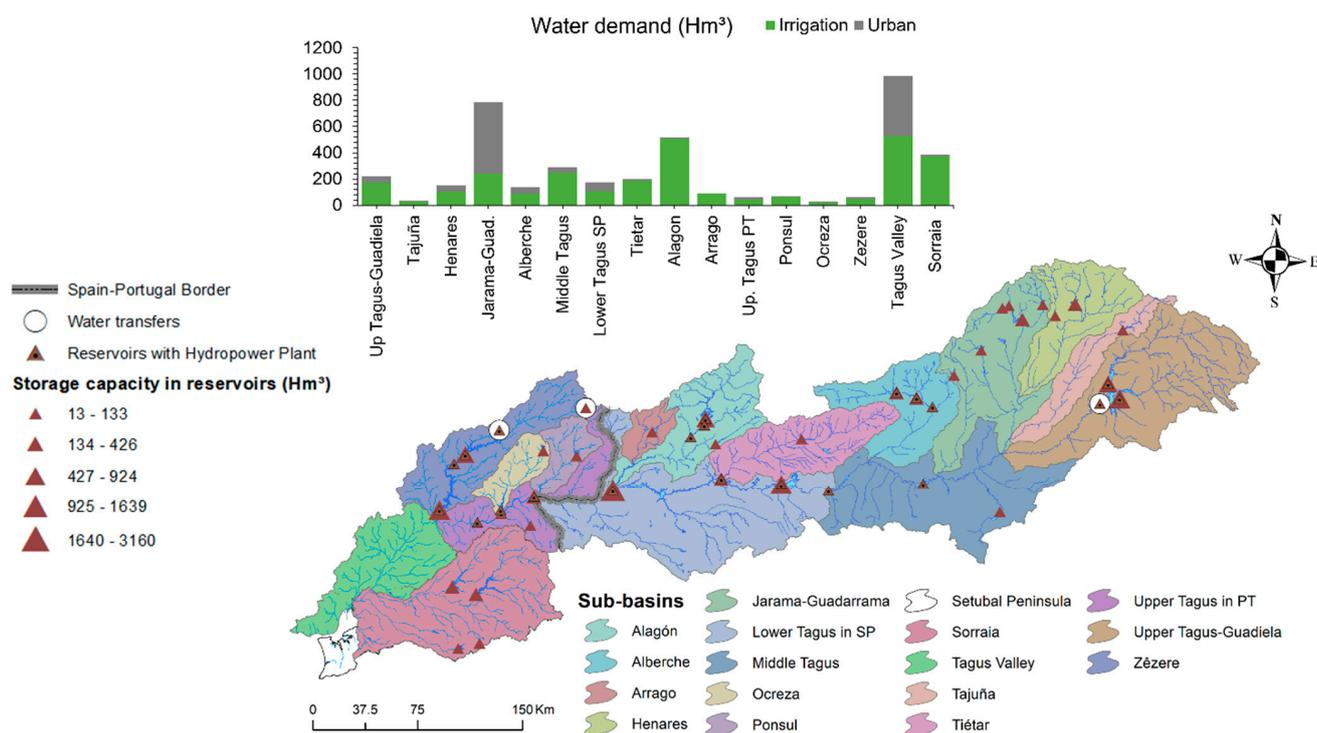
**Figure 1.** Tagus River basin and its human-induced pressures (hydraulic infrastructure and water demand) within sub-basins.
