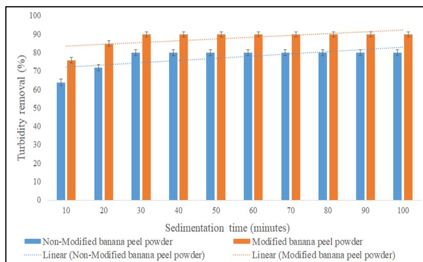
**Figure 5.** Coagulation activity of modified and non-modified banana peel powder at different sedimentation times.
