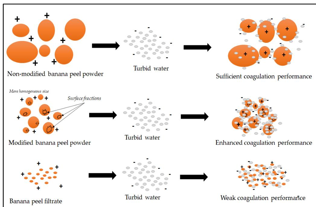
**Figure 8.** Schematic illustration of the coagulation performance of modified and non-modified banana peel powder, and banana peel filtrate.
