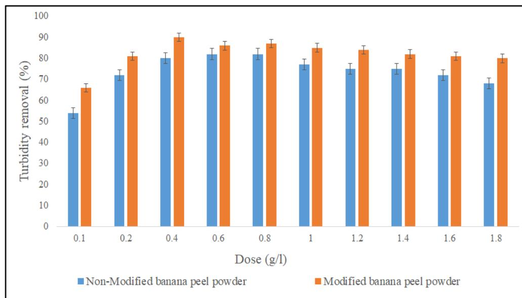
**Figure 3.** Coagulation activity of the modified and non-modified banana peel powder at different doses.
