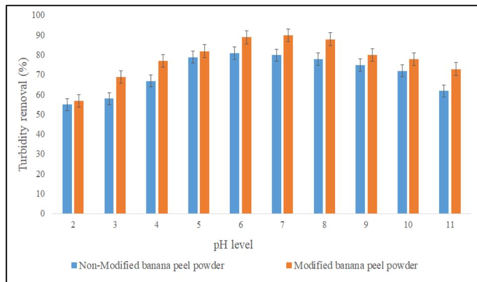
**Figure 4.** Coagulation activity of modified and non-modified banana peel powder at different pH levels.
