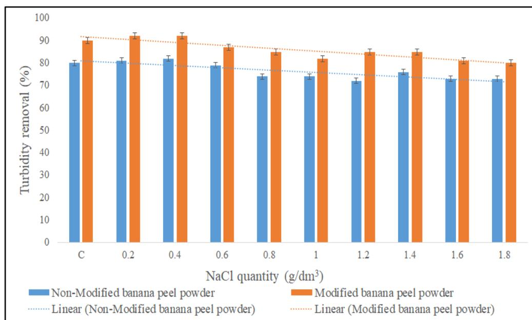
**Figure 6.** Coagulation activity of modified and non-modified banana peel powder at different NaCl quantities.
