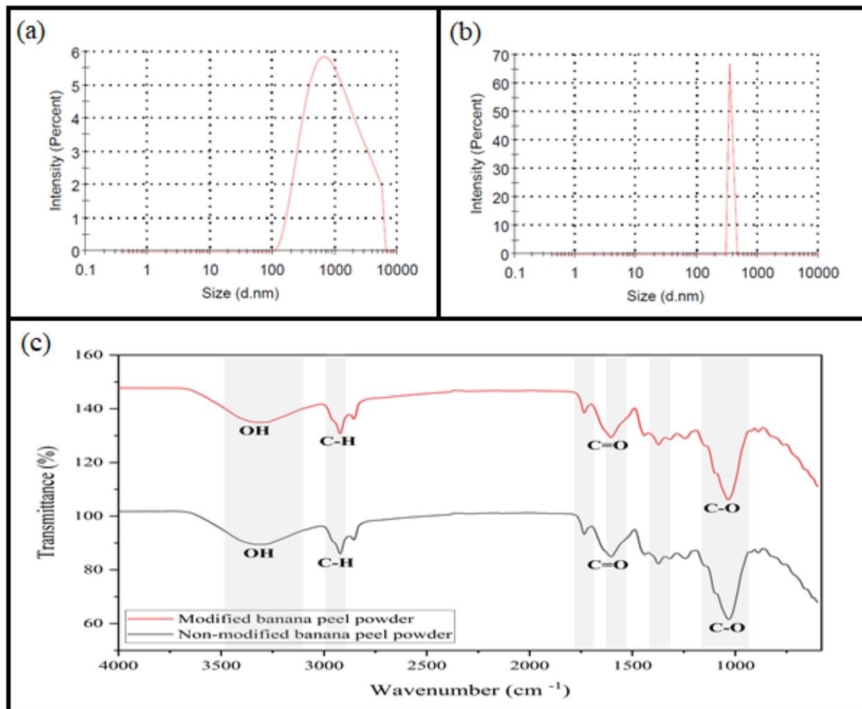
**Figure 2.** Particle size analysis and FT-IR of modified and non-modified banana peel powder; (a,b) average particle size of non-modified and modified banana peel powder, respectively, and (c) FT-IR spectra.
