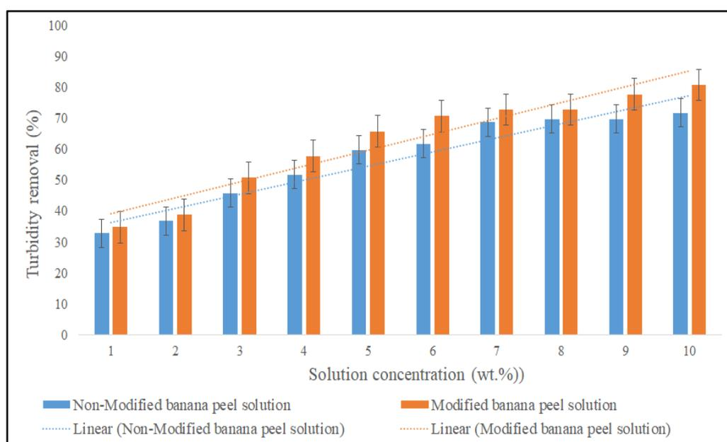
**Figure 7.** Coagulation activity of different concentrations of modified and non-modified banana peel solutions.
