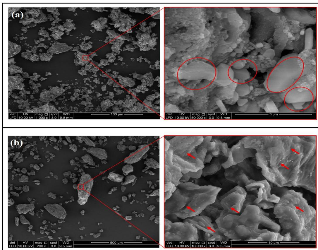
**Figure 1.** Morphological analysis of modified and non-modified banana peel powder; (a) non-modified powder exhibiting smoother surfaces and (b) modified powder exhibiting sticky surfaces, with clear fractions as the arrows indicate.
