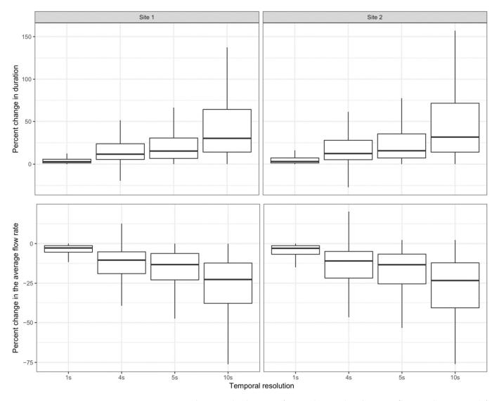
**Figure 4.** Percent change in the duration of events (**top row**) and average flow rate (**bottom row**) for all events at different temporal resolutions compared with events identified from pulse data.
