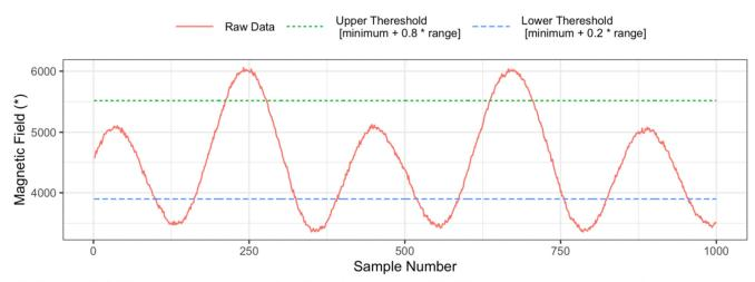
(\*) The magnetic field is expressed as an unsigned number that varies from 0 to 65,535 in the assigned range (± 4 gauss)
