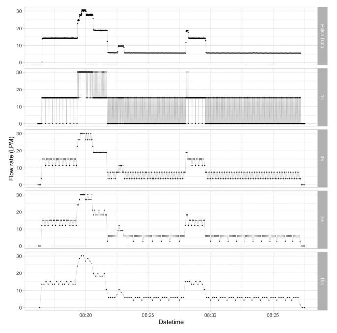
**Figure 10.** Pulse data and time aggregated data converted to flowrates at different temporal resolutions for a single overlapping event at Site 2. Event start date and time: 2022-04-02 08:16:30.910 MT, event duration: 20.6 min.
