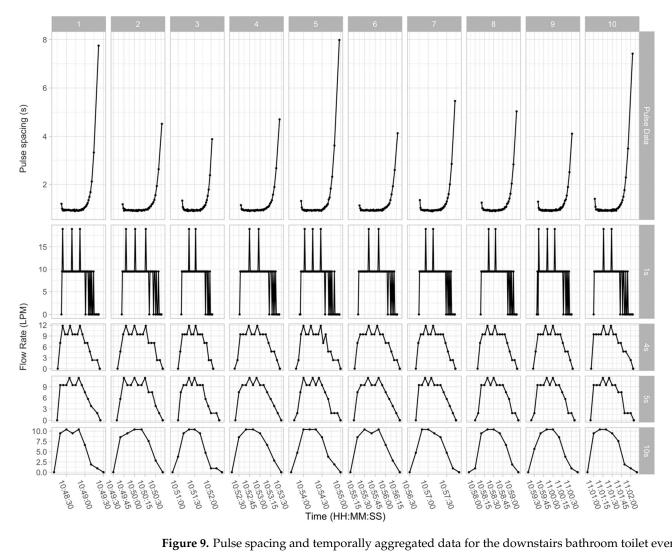
**Figure 9.** Pulse spacing and temporally aggregated data for the downstairs bathroom toilet events from the controlled experiment events at Site 1. Each column (1 to 10) shows a different event.
