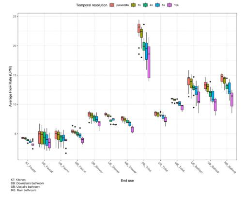
**Figure 5.** Distributions of average flow rate values for the controlled experiment events (Site 1) derived from pulse data and from data aggregated at different temporal resolutions.
