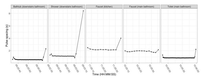
**Figure 3.** Pulse data for different Site 1 events from the controlled experiment. Each panel shows an individual event. The first value of each event was removed for visualization as it represents time since the previous event.
